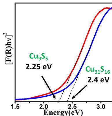
Fig. 6 Plots of  $[F(R)hv]^2$  vs. energy (eV) generated by Kubelka–Munk transformation of solid-state diffuse reflectance data of  $\text{Cu}_9\text{S}_5$  and  $\text{Cu}_{31}\text{S}_{16}$  nanoparticles.
