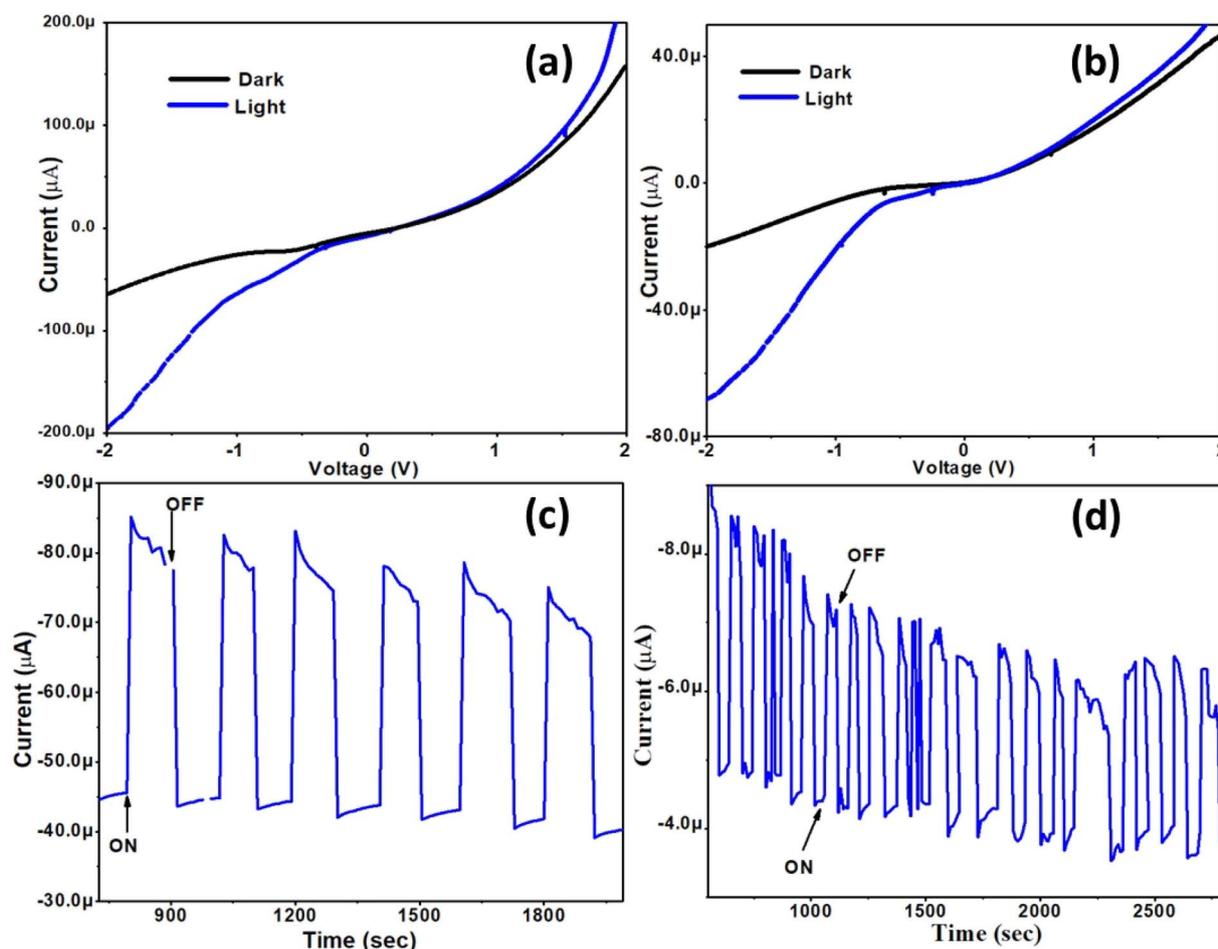
Fig. 7 (a and b)  $I$ - $V$  characteristics and (c and d) switching behaviour under alternating light and dark conditions for  $\text{Cu}_9\text{S}_5$  and  $\text{Cu}_{31}\text{S}_{16}$  nanoparticles.
