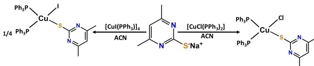
Scheme 1 Synthesis of [CuCl(dmpymSH)(PPh<sub>3</sub>)<sub>2</sub>] (1) and [CuI(dmpymSH)(PPh<sub>3</sub>)<sub>2</sub>] (2).
