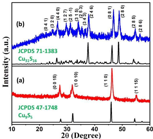
Fig. 3 XRD profiles of copper sulfide nanostructures obtained via the thermolysis of (a)  $[\text{CuCl}(\text{dmpymSH})(\text{PPh}_3)_2]$  (**1**) and (b)  $[\text{Cu}(\text{dmpymSH})(\text{PPh}_3)_2]$  (**2**).
