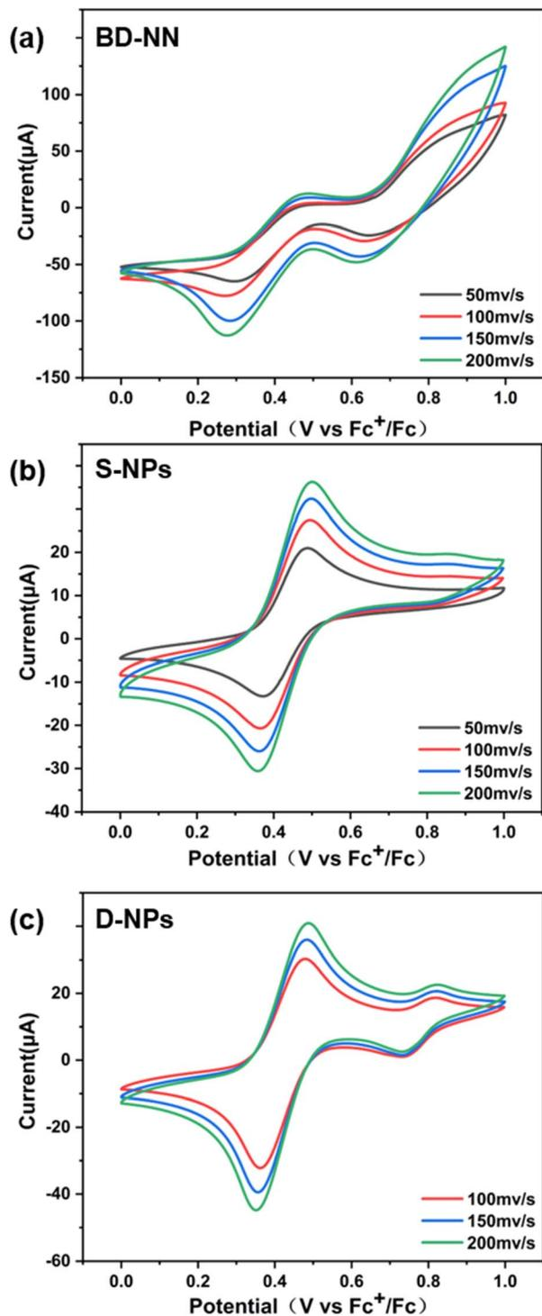
Fig. 5 (a) CV spectrum of BD-NN; (b) CV spectrum of S-NPs; (c) CV spectrum of D-NPs. Each set of tests adopts  $50 \text{ mV s}^{-1}$ ,  $100 \text{ mV s}^{-1}$ ,  $150 \text{ mV s}^{-1}$ , and  $200 \text{ mV s}^{-1}$  sweep speeds. The CVs were all tested in  $\text{CH}_3\text{CN}$  with  $0.02 \text{ M}$  tetrabutylammonium hexafluorophosphate as electrolyte and Pt as working electrode.
