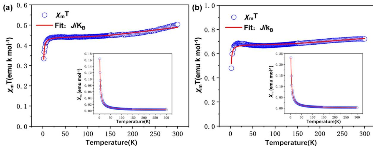
Fig. 9 SQUID magnetometry of solid samples: plots of  $\chi_m T$  vs.  $T$  at  $H = 10\,000.31543$  Oe in the warming mode (blue circle). Inset plots:  $\chi_m$  vs.  $T$  in the warming mode and fitting (solid red line) curves of (a) S-NPs; (b) D-NPs. The drawing data is subtracted from the background.
