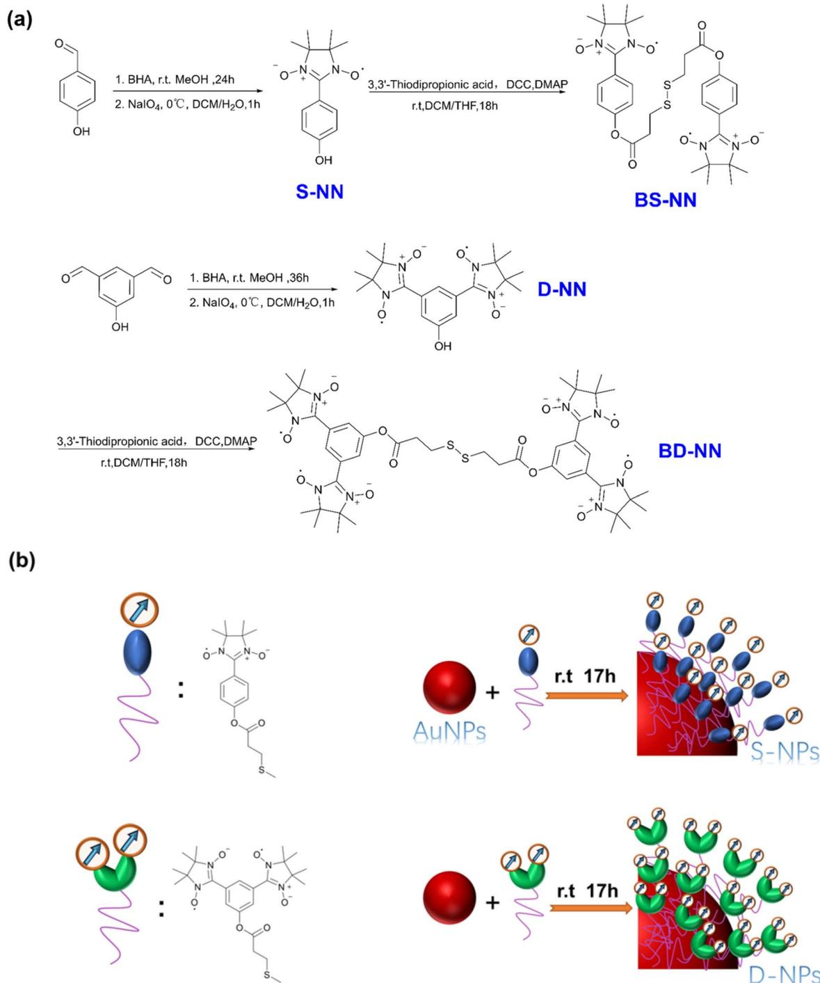
Fig. 1 (a) Synthesis flow chart of S-NN, BS-NN, D-NN and BD-NN; (b) composite concept diagram of S-NPs and D-NPs. The red ball refers to triocetylamine stabilized gold nanoparticles.
