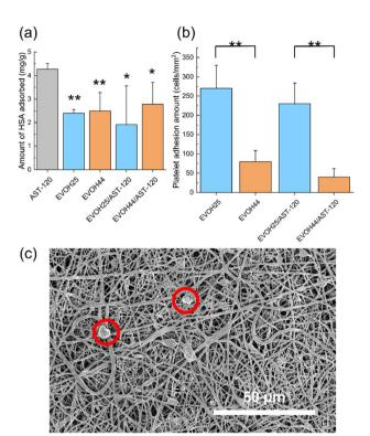
Fig. 6 (a) Amount of human serum albumin adsorbed by the AST-120 powder and nanofibers. (Mean  $\pm$  SD, n=3, \*p<0.05, \*\*p<0.01). (b) Amount of platelet adhesion to nanofibers, as assessed based on the FE-SEM image. (Mean  $\pm$  SD, n=10, \*\*p<0.01). (c) FE-SEM image of platelets adhering onto the EVOH25/AST-120 nanofibers.
