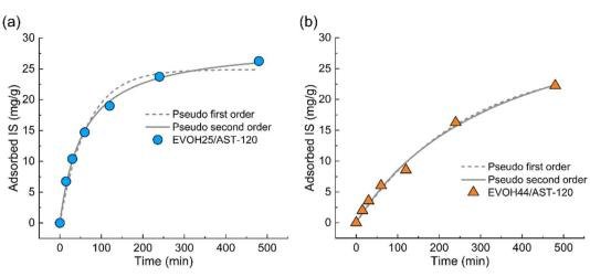
Fig. 5 Pseudo-first-order model and pseudo-second-order model of IS adsorption by (a) EVOH25/AST-120 nanofibers and (b) EVOH44/AST-120 nanofibers.
