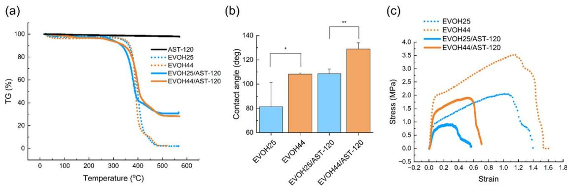
Fig. 3 (a) TG-DTA curve of the AST-120 powder, EVOH nanofibers, and EVOH/AST-120 nanofibers. (b) Water contact angles on the surface of the EVOH nanofibers and EVOH/AST-120 nanofibers. (Mean  $\pm$  SD,  $n = 3$ , \* $p < 0.05$ , \*\* $p < 0.01$ ). (c) Stress–strain curves of EVOH nanofibers and EVOH/AST-120 nanofibers.
