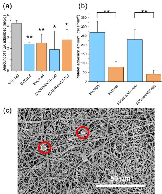
Fig. 6 (a) Amount of human serum albumin adsorbed by the AST-120 powder and nanofibers. (Mean  $\pm$  SD,  $n = 3$ ,  $*p < 0.05$ ,  $**p < 0.01$ ). (b) Amount of platelet adhesion to nanofibers, as assessed based on the FE-SEM image. (Mean  $\pm$  SD,  $n = 10$ ,  $**p < 0.01$ ). (c) FE-SEM image of platelets adhering onto the EVOH25/AST-120 nanofibers.
