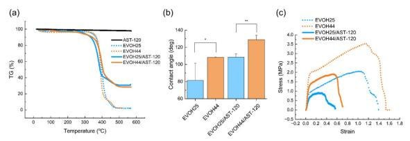
Fig. 3 (a) TG-DTA curve of the AST-120 powder, EVOH nanofibers, and EVOH/AST-120 nanofibers. (b) Water contact angles on the surface of the EVOH nanofibers and EVOH/AST-120 nanofibers. (Mean  $\pm$  SD, n=3, \*p<0.05, \*\*p<0.01). (c) Stress-strain curves of EVOH nanofibers and EVOH/AST-120 nanofibers.
