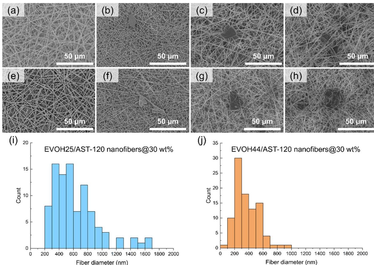
**Fig. 1** (a–h): FE-SEM images of the EVOH nanofibers and EVOH/AST-120 nanofibers. The ethylene ratio of EVOH was (a–d) 25 mol% and (e–h) 44 mol%. The content ratio of AST-120 used in the preparation was (a and e) 0 wt%, (b and f) 10 wt%, (c and g) 20 wt%, and (d and h) 30 wt%. (i and j): histogram of fiber diameter of EVOH25/AST-120 and EVOH44/AST-120 nanofibers respectively ( $n = 60$ ). The content ratio of AST-120 was 30 wt%.
