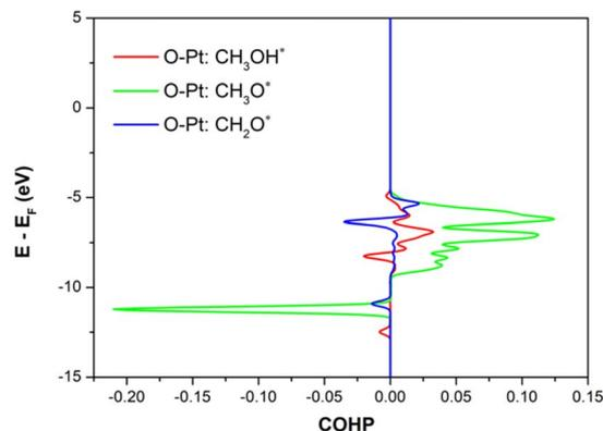
Fig. 6 The crystal orbital Hamilton population of the O–Pt bonding interaction between the intermediates ( $\text{CH}_3\text{OH}^*$ ,  $\text{CH}_3\text{O}^*$ , and  $\text{CH}_2\text{O}^*$ ) and the  $\text{PtRuCo}_3/\text{C-MWCNT}$  substrate.
