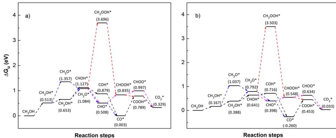
Fig. 7 Gibbs free energy diagram for the methanol oxidation reaction on (a) PtRuFe<sub>3</sub>/C-MWCNT and (b) PtRuCo<sub>3</sub>/C-MWCNT substrates at an applied potential ( $U$ ) of 0 V, a pressure of 1 bar, and a temperature of 300 K. For simplicity, the hydrogen and water molecules in each step have been omitted in the diagrams. Relative Gibbs free energy (eV) is in parenthesis.
