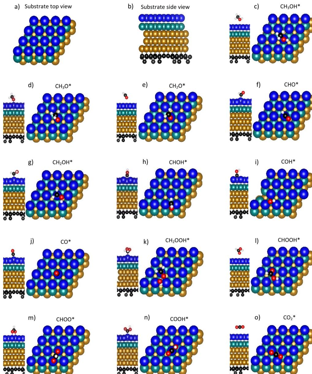
Fig. 1 The top and side views of the substrates (a and b) and the most stable configurations for the adsorption of methanol oxidation intermediates on the surface of PtRuM<sub>3</sub>/C-MWCNTs (M = Fe and Co) catalysts (c–o). Topmost-layer Pt (blue), Ru (green), Fe (golden), C (black), O (red), and H (white).
