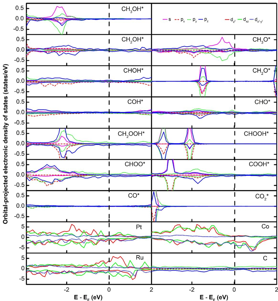
Fig. 4 The orbital-projected electronic density of states for the systems of the PtRuCo<sub>3</sub>/C-MWCNT substrate and the adsorbed intermediate:  $d_{xz}$  is identical to  $d_{yz}$ , and  $d_{xy}$  is identical to  $d_{x^2-y^2}$ . For the PtRuFe<sub>3</sub>/C-MWCNT substrate, see Fig. S2 in ESI.†
