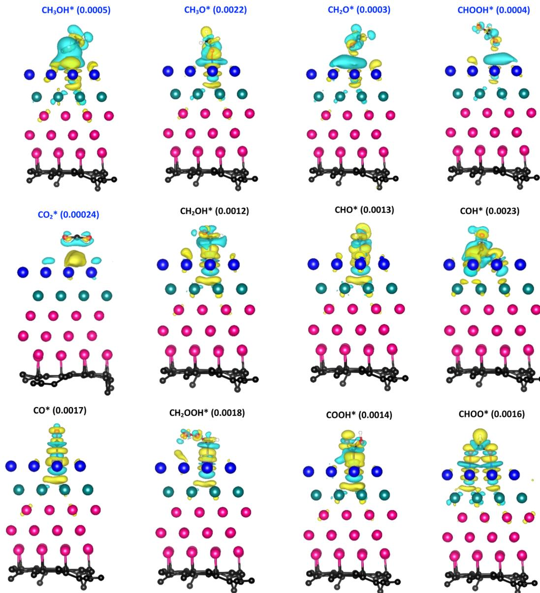
Fig. 5 The charge density difference of the systems of the adsorbed intermediate on the PtRuCo<sub>3</sub>/C-MWCNT substrate. The isosurface values are inside parentheses, with the unit being e<sup>-</sup> Å<sup>-3</sup>.
