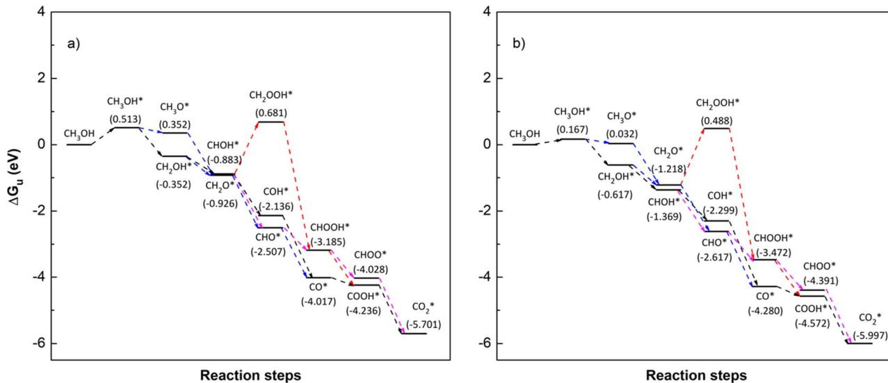
Fig. 8 Gibbs free energy diagram for the methanol oxidation reaction on (a) PtRuFe<sub>3</sub>/C-MWCNT and (b) PtRuCo<sub>3</sub>/C-MWCNT substrates at an applied potential ( $U$ ) of 1.005 V, pressure of 1 bar, and temperature of 300 K. For simplicity, the hydrogen and water molecules in the reaction equations have been omitted in the diagrams. Relative Gibbs free energy (eV) is in parenthesis.
