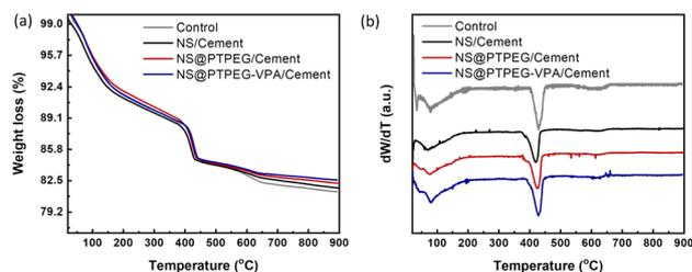
Fig. 8 (a) TGA curves and (b) differential TGA curves under the addition of 0.8 wt% pristine and modified NS at 72 h.
