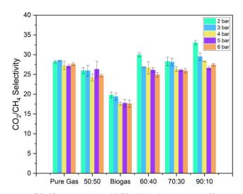
Fig. 21  $CO_2/CH_4$  selectivity of DZ5 MMMs for mixed gas (CH $_4$  and  $CO_2$ ) in different ratios. Pure gas results are also shown for comparison.
