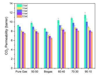
Fig. 19  $CO_2$  permeability of DZ5 MMMs for mixed gas (CH<sub>4</sub> and CO<sub>2</sub>) in different ratios (shown in x-axis are CH<sub>4</sub>:  $CO_2$  ratio). Pure gas results are also shown for comparison.
