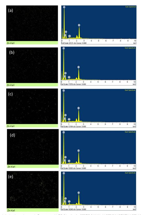
Fig. 4 EDS analysis showing an increase in Zn content with ZIF-8 loading for PSF/ZIF-8 MMMs (a) DZ0.5 (b) DZ0.75 (c) DZ1 (d) DZ2 (e) DZ5.
