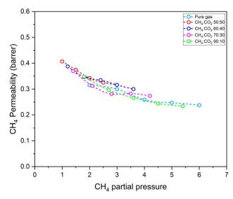
Fig. 14  $\,$  CH $_4$  permeability of pure PSF membranes for mixed gas (CH $_4$  and CO $_2$ ) in different ratios. Pure gas results are also shown for comparison.
