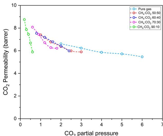
Fig. 13  $\text{CO}_2$  permeability of pure PSF membranes for mixed gas ( $\text{CH}_4$  and  $\text{CO}_2$ ) in different ratios. Pure gas results are also shown for comparison.
