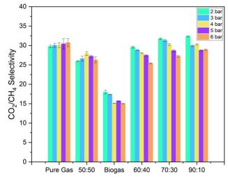
Fig. 18  $CO_2/CH_4$  selectivity of DZ1 MMMs for mixed gas (CH<sub>4</sub> and  $CO_2$ ) in different ratios (shown in x-axis are  $CH_4$ :  $CO_2$  ratio). Pure gas results are also shown for comparison.
