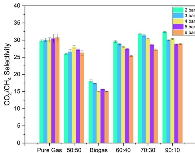
Fig. 18 CO<sub>2</sub>/CH<sub>4</sub> selectivity of DZ1 MMMs for mixed gas (CH<sub>4</sub> and CO<sub>2</sub>) in different ratios (shown in x-axis are CH<sub>4</sub> : CO<sub>2</sub> ratio). Pure gas results are also shown for comparison.
