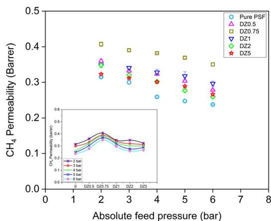
Fig. 9  $\text{CH}_4$  permeability of dense PSF/ZIF-8 mixed matrix membranes at different loadings of ZIF-8. Pure PSF results are also shown for comparison. Inset shows the permeabilities plotted as a function of loading for different pressures.
