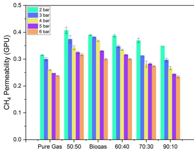
Fig. 12  $\text{CH}_4$  permeability of pure PSF membranes for mixed gas ( $\text{CH}_4$  and  $\text{CO}_2$ ) in different ratios (shown in x-axis are  $\text{CH}_4 : \text{CO}_2$  ratio). Pure gas results are also shown for comparison.
