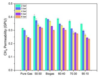
Fig. 12  $CH_4$  permeability of pure PSF membranes for mixed gas ( $CH_4$  and  $CO_2$ ) in different ratios (shown in x-axis are  $CH_4$ :  $CO_2$  ratio). Pure gas results are also shown for comparison.
