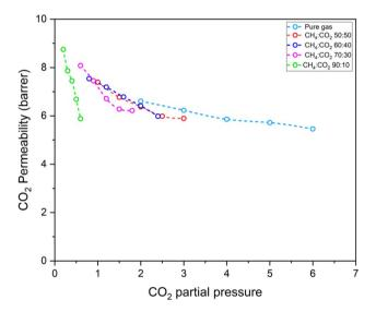
Fig. 13  $CO_2$  permeability of pure PSF membranes for mixed gas (CH<sub>4</sub> and  $CO_2$ ) in different ratios. Pure gas results are also shown for comparison.
