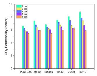
Fig. 11  $CO_2$  permeability of pure PSF membranes for mixed gas (CH<sub>4</sub> and CO<sub>2</sub>) in different ratios (shown in *x*-axis are CH<sub>4</sub>: CO<sub>2</sub> ratio). Pure gas results are also shown for comparison.
