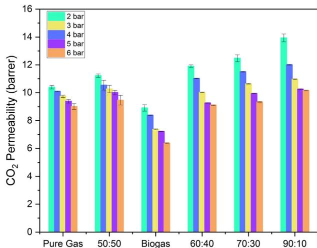
Fig. 16 CO<sub>2</sub> permeability of DZ1 MMMs for mixed gas (CH<sub>4</sub> and CO<sub>2</sub>) in different ratios (shown in x-axis are CH<sub>4</sub> : CO<sub>2</sub> ratio). Pure gas results are also shown for comparison.
