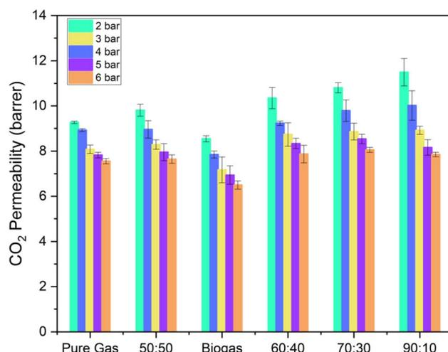
Fig. 19 CO<sub>2</sub> permeability of DZ5 MMMs for mixed gas (CH<sub>4</sub> and CO<sub>2</sub>) in different ratios (shown in x-axis are CH<sub>4</sub> : CO<sub>2</sub> ratio). Pure gas results are also shown for comparison.
