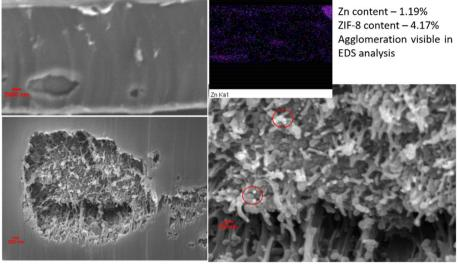
Fig. 6 Cross sectional micrographs of DZ2 membrane showing agglomeration and EDS analysis showing ZIF-8 particles agglomeration (red circles)
