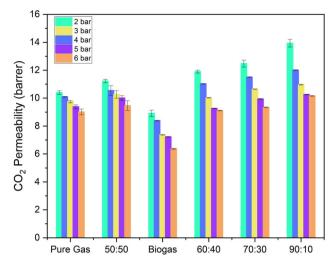
Fig. 16  $CO_2$  permeability of DZ1 MMMs for mixed gas (CH<sub>4</sub> and CO<sub>2</sub>) in different ratios (shown in x-axis are CH<sub>4</sub> : CO<sub>2</sub> ratio). Pure gas results are also shown for comparison.
