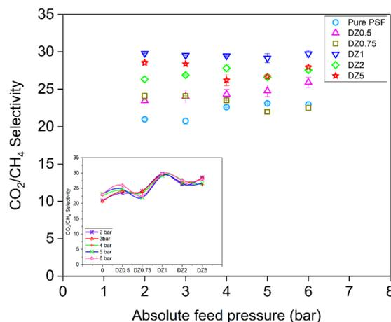
Fig. 10  $\text{CO}_2/\text{CH}_4$  selectivity of dense PSF/ZIF-8 mixed matrix membranes at different loadings of ZIF-8. Pure PSF results are also shown for comparison. Inset shows the selectivity plotted as a function of loading for different pressures.
