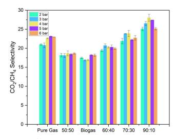
Fig. 15  $CO_2/CH_4$  selectivity of pure PSF membranes for mixed gas  $(CH_4 \text{ and } CO_2)$  in different ratios (shown in x-axis are  $CH_4$ :  $CO_2$  ratio). Pure gas results are also shown for comparison.
