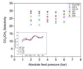
Fig. 10  $\rm CO_2/CH_4$  selectivity of dense PSF/ZIF-8 mixed matrix membranes at different loadings of ZIF-8. Pure PSF results are also shown for comparison. Inset shows the selectivity plotted as a function of loading for different pressures.
