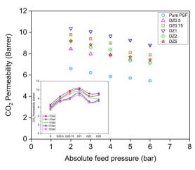
Fig. 8  $\rm CO_2$  permeability of dense PSF/ZIF-8 mixed matrix membranes at different loadings of ZIF-8. Pure PSF results are also shown for comparison. Inset shows the permeabilities plotted as a function of loading for different pressures.
