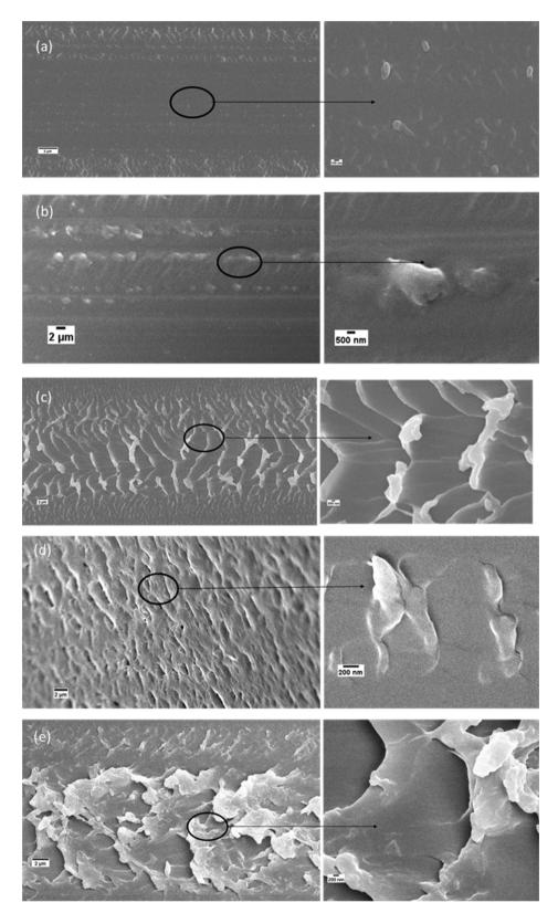
Fig. 5 SEM micrographs (cross section) for dense PSF/ZIF-8 mixed matrix membranes (a) DZ0.5 (b) DZ0.75 (c) DZ1 (d) DZ2 (e) DZ5. The panels on the right show the circled regions from the corresponding panels on the left at a higher magnification.
