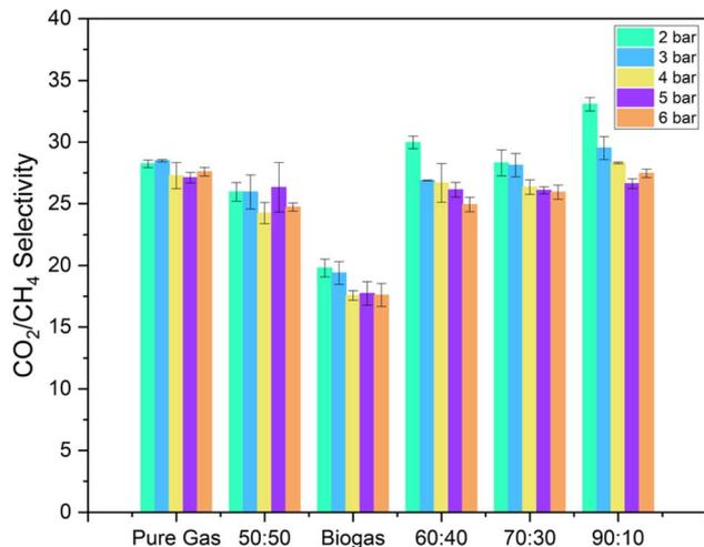
Fig. 21 CO<sub>2</sub>/CH<sub>4</sub> selectivity of DZ5 MMMs for mixed gas (CH<sub>4</sub> and CO<sub>2</sub>) in different ratios. Pure gas results are also shown for comparison.
