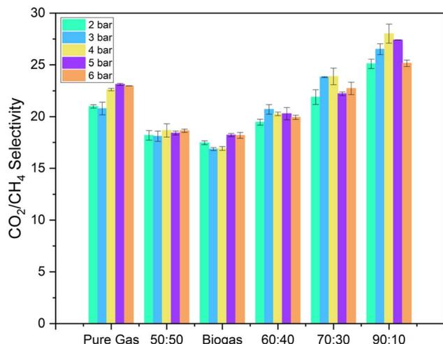
Fig. 15  $\text{CO}_2/\text{CH}_4$  selectivity of pure PSF membranes for mixed gas ( $\text{CH}_4$  and  $\text{CO}_2$ ) in different ratios (shown in x-axis are  $\text{CH}_4 : \text{CO}_2$  ratio). Pure gas results are also shown for comparison.
