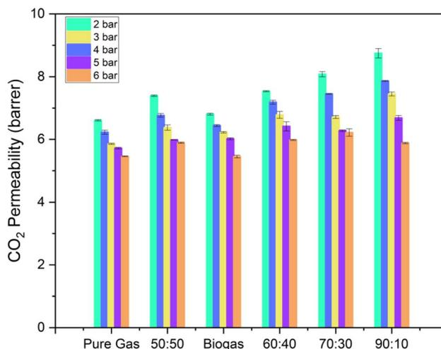
Fig. 11  $\text{CO}_2$  permeability of pure PSF membranes for mixed gas ( $\text{CH}_4$  and  $\text{CO}_2$ ) in different ratios (shown in x-axis are  $\text{CH}_4 : \text{CO}_2$  ratio). Pure gas results are also shown for comparison.
