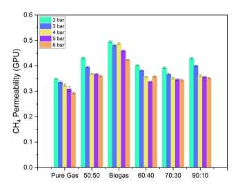
Fig. 17 CH<sub>4</sub> permeability of DZ1 MMMs for mixed gas (CH<sub>4</sub> and CO<sub>2</sub>) in different ratios (shown in x-axis are CH<sub>4</sub>: CO<sub>2</sub> ratio). Pure gas results are also shown for comparison.
