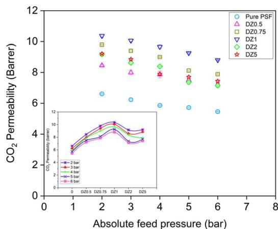
Fig. 8  $\text{CO}_2$  permeability of dense PSF/ZIF-8 mixed matrix membranes at different loadings of ZIF-8. Pure PSF results are also shown for comparison. Inset shows the permeabilities plotted as a function of loading for different pressures.
