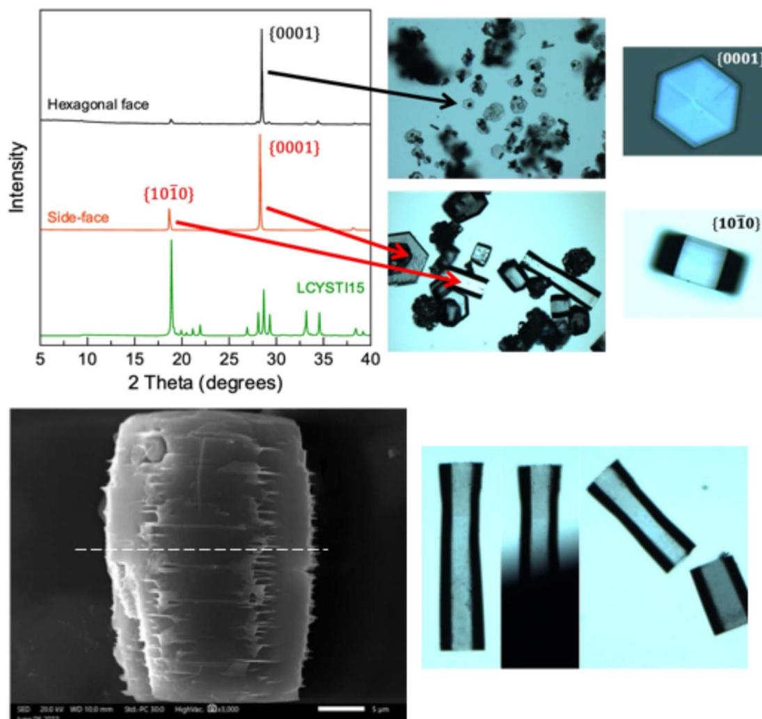
Fig. 3 Cystine crystals face indexed by a combination of observation in a light microscope and X-ray diffraction of that preferential orientation via PXRD, magnification,  $\times 4$ . The way in which cystine crystals grow create fractures apparent at the vertex between two  $\{10\bar{1}0\}$  edges, this may result in a vulnerability to pressure normal to this face, causing cleavage. SEM scale = 5  $\mu\text{m}$ .
