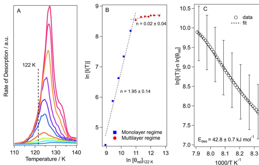
Fig. 6 (A) TPD traces of increasing exposures ( $2 L_m$  to  $100 L_m$ ) of methyl acetate ice desorption from an HOPG surface. (B) Order of desorption plot constructed from the QMS signal intensity at 122 K from the data in panel (A). (C) Multilayer desorption energy plot for the  $50 L_m$  data in panel (A).
