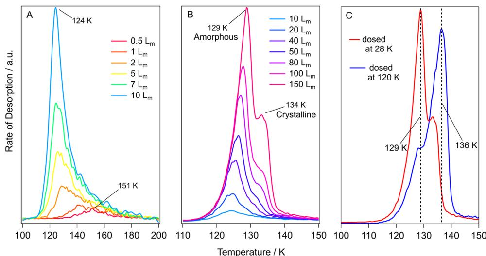
**Fig. 4** TPD spectra for varying exposures of methyl acetate adsorbed on HOPG. (A) Exposures from 0.5  $L_{\text{m}}$ –10  $L_{\text{m}}$  dosed at 28 K. (B) Exposures from 10  $L_{\text{m}}$ –150  $L_{\text{m}}$  dosed at 28 K. (C) A comparison of 150  $L_{\text{m}}$  methyl acetate ices grown at 28 K and 120 K.
