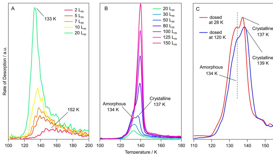
Fig. 5 TPD data for varying exposures of methyl propanoate adsorbed on HOPG. (A) Exposures from 2  $L_m$ –20  $L_m$  dosed at 28 K. (B) Exposures from 20  $L_m$ –150  $L_m$  dosed at 28 K. (C) A comparison of 50  $L_m$  methyl propanoate ices grown at 28 K and 120 K.
