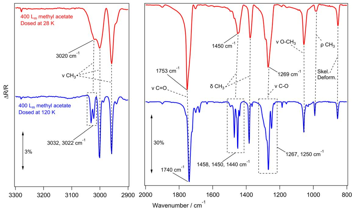
Fig. 2 Experimental RAIR spectra of 400  $L_m$  methyl acetate adsorbed on HOPG at 28 K (red) and 120 K (blue). Selected vibrational modes are highlighted in the spectra. The left hand panel shows the 2900–3300  $\text{cm}^{-1}$  wavenumber region and the right hand panel shows the region from 800–2000  $\text{cm}^{-1}$ . No vibrational bands are seen in other regions of the spectrum.
