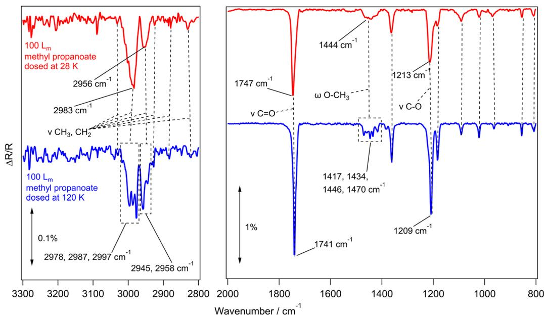
Fig. 3 RAIR spectra of 100 L<sub>m</sub> methyl propanoate adsorbed on HOPG at 28 K (red) and 120 K (blue). Selected vibrational modes are highlighted in the spectra. The left hand panel shows the 2800–3300 cm<sup>-1</sup> wavenumber region and the right hand panel shows the region from 800–2000 cm<sup>-1</sup>. No vibrational bands are seen in other regions of the spectrum.
