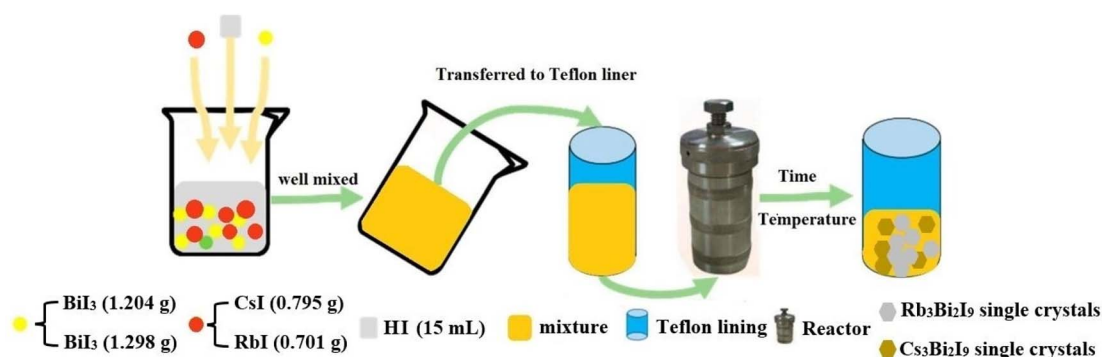
Fig. 1 Unveiling the solvothermal route to \text{A}_3\text{Bi}_2\text{I}_9 ( \text{A} = \text{Cs}, \text{Rb} ) single crystals: a schematic depiction.
