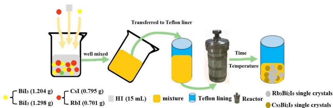
Fig. 1 Unveiling the solvothermal route to \text{A}_3\text{Bi}_2\text{I}_9 ( \text{A} = \text{Cs, Rb} ) single crystals: a schematic depiction.
