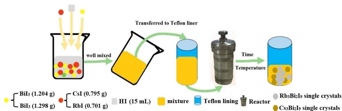
Fig. 1 Unveiling the solvothermal route to \text{A}_3\text{Bi}_2\text{I}_9 ( \text{A} = \text{Cs}, \text{Rb} ) single crystals: a schematic depiction.
