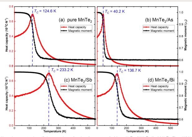
Fig. 6 Magnetic moment and specific heat capacity as a function of temperature for (a) pure  $MnTe_2$ , (b)  $MnTe_2/As$ , (c)  $MnTe_2/Sb$  and (d)  $MnTe_2/Bi$  via Monte Carlo simulations.
