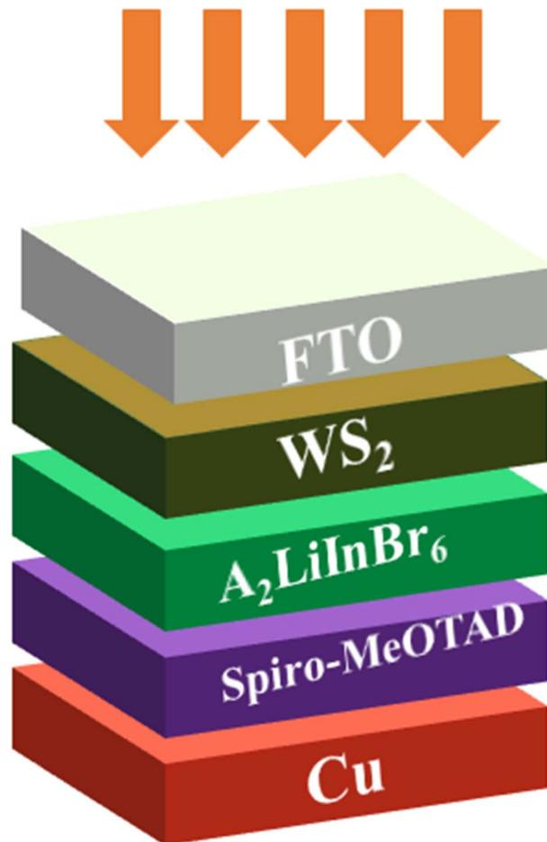
Fig. 5 Schematic diagram of the solar cell device having  $A_2LiInBr_6$  ( $A = Rb, Cs$ ) lead free halide perovskites as a active layer.
