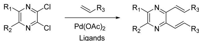
Fig. 2 The synthesis of 2,3-dialkenyl-substituted quinoxalines via the Heck method.
