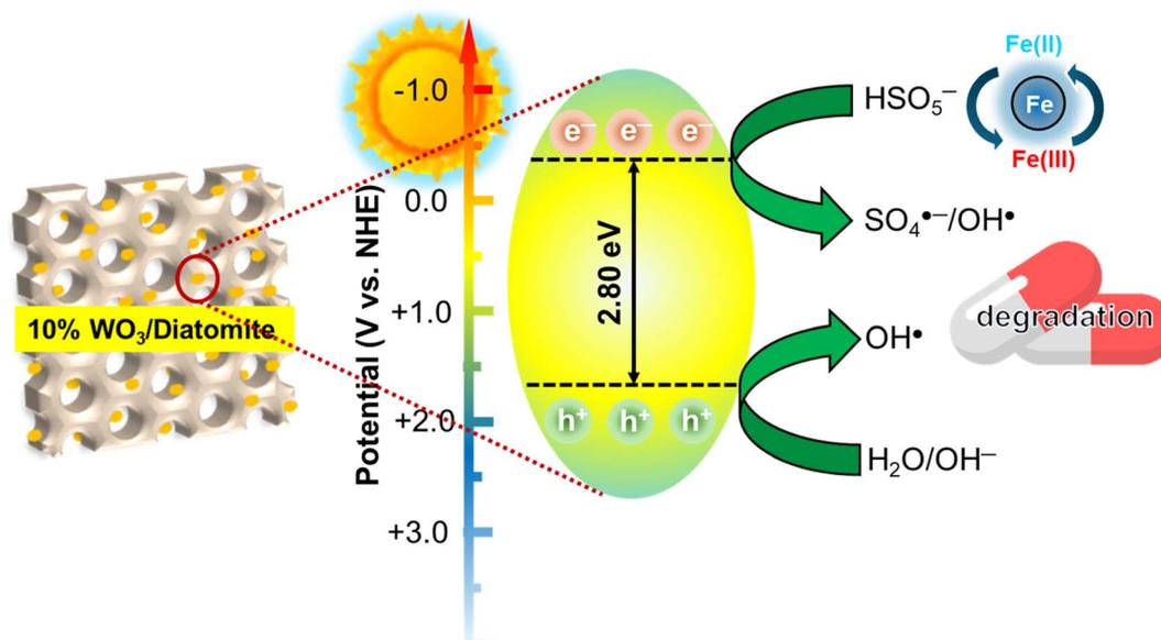
Fig. 8 Proposed photocatalytic tetracycline degradation of 10% WO<sub>3</sub>/diatomite composites in coupling with PMS activation under visible light.
