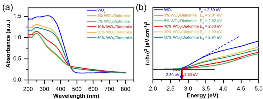
Fig. 5 DRS spectra of the as-prepared materials (a) and estimated band gap of WO<sub>3</sub> and 10% WO<sub>3</sub>/diatomite composite (b).
