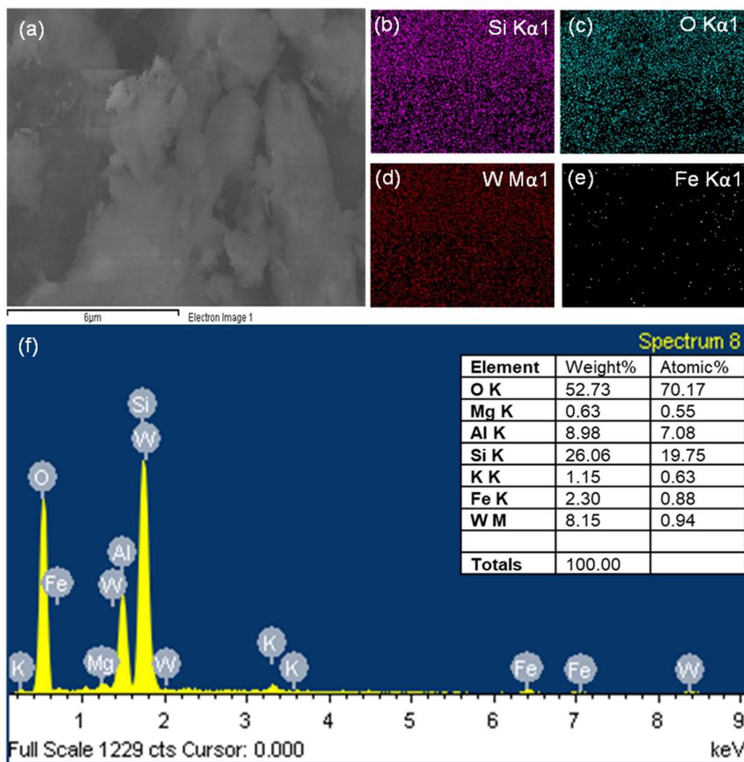
Fig. 4 SEM of 10% WO<sub>3</sub>/diatomite (a), elemental mapping (b–e) and EDS spectrum of 10% WO<sub>3</sub>/diatomite (f).
