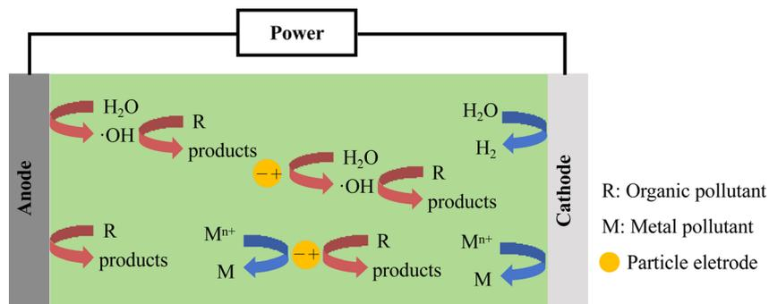
Fig. 4 General electrocatalysis mechanism in a 3D-ER.
