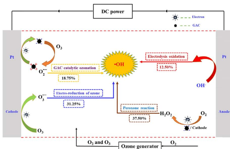
Fig. 9 Possible degradation mechanism of NB by GAC in 3D-ER/O<sub>3</sub>. Reproduced from ref. 45 with permission from [Elsevier], copyright [2020].
