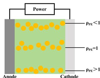
Fig. 3 3D-ER with particle electrodes of different densities.
