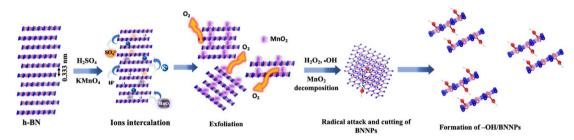
Fig. 1 Schematic representation of the synthesis mechanism of -OH/BNNPs
