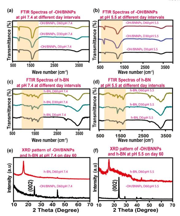
Fig. 5 FTIR spectra of -OH/BNNPs after treatment (a) at pH 7.4 ( $D_0-D_{60}$ ) and (b) pH 5.5 ( $D_0-D_{60}$ ). FTIR spectra of h-BN after treatment (c) at pH 7.4 ( $D_0-D_{60}$ ) and (d) pH 5.5 ( $D_0-D_{60}$ ). XRD pattern of -OH/BNNPs and h-BN after treatment (e) at pH 7.4 ( $D_{60}$ ) and (f) pH 5.5 ( $D_{60}$ ).
