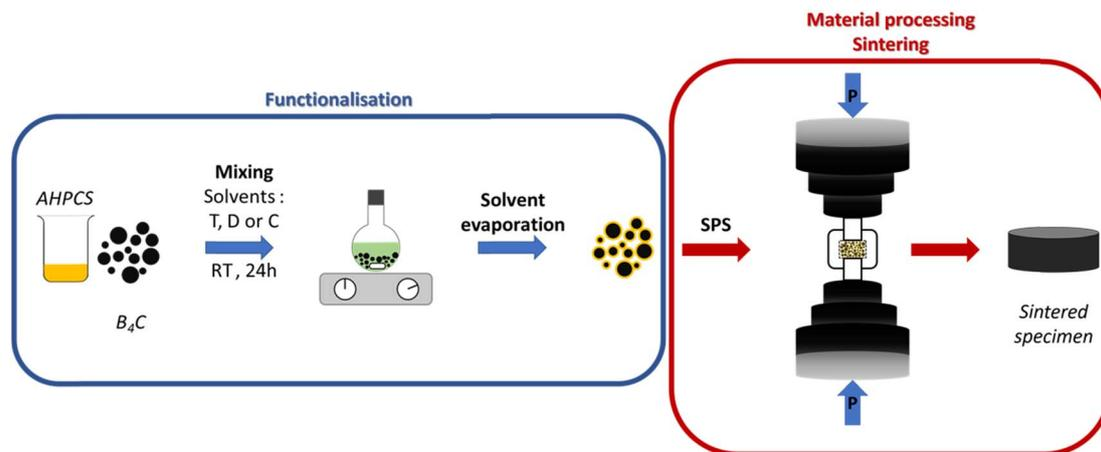
Fig. 2 General protocol for the functionalisation of the B<sub>4</sub>C particle with AHPCS, followed by sintering (T = toluene; D = diethyl ether; C = cyclopentane).
