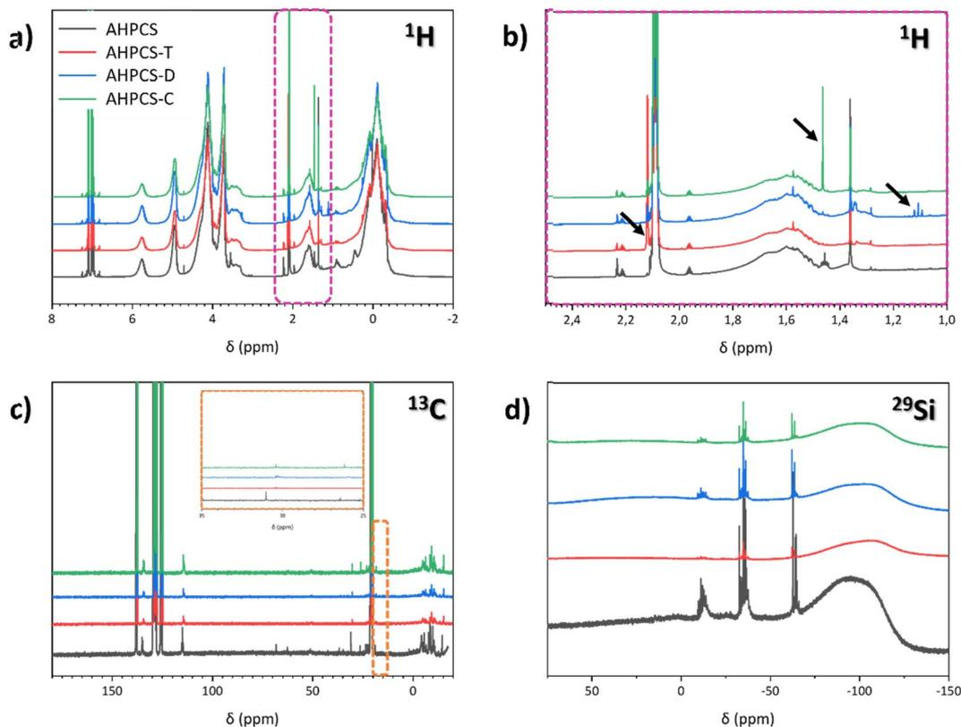
Fig. 5 <sup>1</sup>H (a and b), <sup>13</sup>C (c), and <sup>29</sup>Si (d) NMR analysis of the AHPCS before and after being dissolved in T, D and C.
