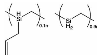
**Fig. 1** AHPCS (SMP-10, Starfire Systems) structure confirmed by the literature.<sup>14</sup>
