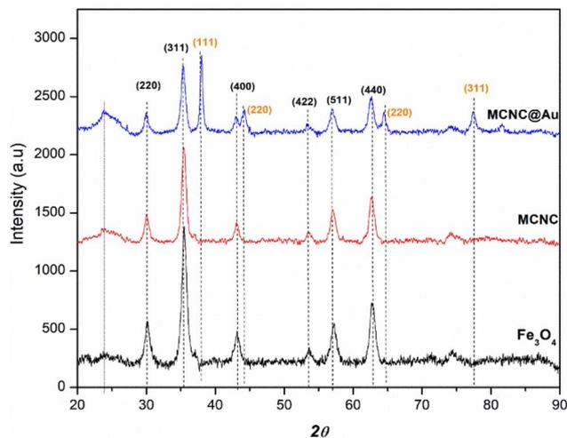
Fig. 7 P-XRD patterns of  $\text{Fe}_3\text{O}_4$ , MCNC and MCNC@Au.
