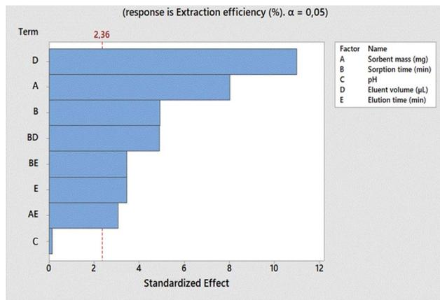
Fig. 9 2-Level  $\frac{1}{2}$  fractional factorial design Pareto chart ( $n = 3$ ) of total sulfur removal for the optimization of mass of sorbent, sorbent time, pH, eluent volume and elution time at 95% confidence level.
