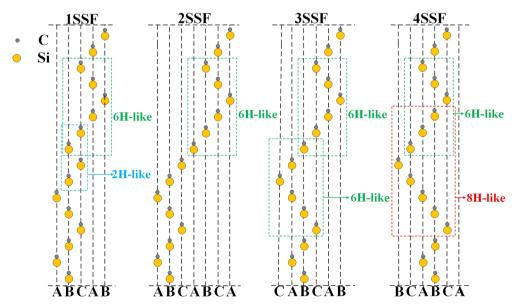
Fig. 4 The structural differences of different SSF viewed from direction [1120].
