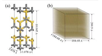
(a) Unitcell of 4H-SiC and (b) supercell of 4H-SiC.
