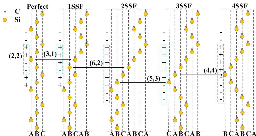
Fig. 1 SSF of 4H-SiC viewed from direction  $[11\bar{2}0]$ .
