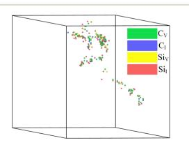
Fig. 9 Irradiation displacement cascade in perfect 4H-SiC.
