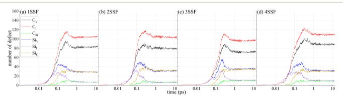
Fig. 6 Time evolution of the number of defect in the displacement cascade of 4H-SiC with one (a) 1SSF, (b) 2SSF, (c) 3SSF, and (d) 4SSF.
