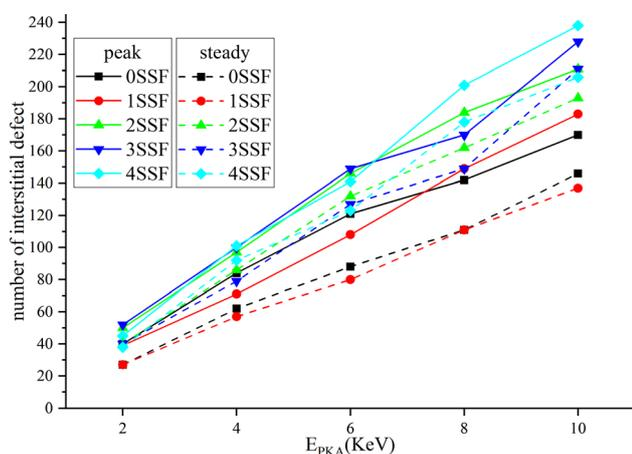
Fig. 11 Relationship curve between the number of defects and  $E_{\text{PKA}}$ .
