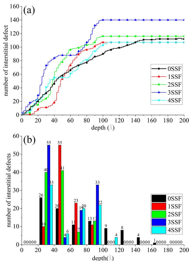
Fig. 10 Relationship between the number of defects and incident depth. (a) Curve between the number of defects and incident depth; (b) defect quantity within the range of every 20 Å.
