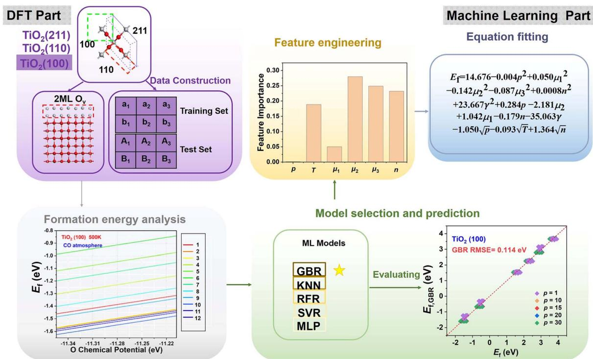
**Scheme 1** The ML workflow. The optimized geometry of  $\text{TiO}_2(100)$  after removing the O atoms from the first two layers is shown in purple. The gray box denotes the database construction. The green boxes show the model selection and prediction phases of this work. The yellow box represents the feature engineering stage. The blue part represents the equation fitting process.
