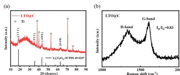
Fig. 1 XRD pattern and Raman spectra of LTO@C. (a) the XRD pattern, and (b) the Raman spectra.
