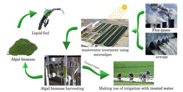
Fig. 1 Typical algae-based wastewater treatment.
