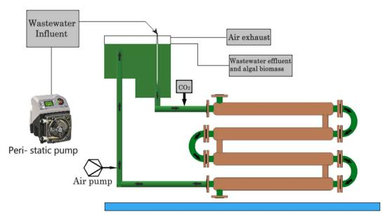
Fig. 7 Lab-scale closed photobioreactor for pollutant removal.
