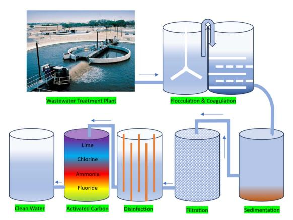
Fig. 4 Stages in wastewater treatment plant.
