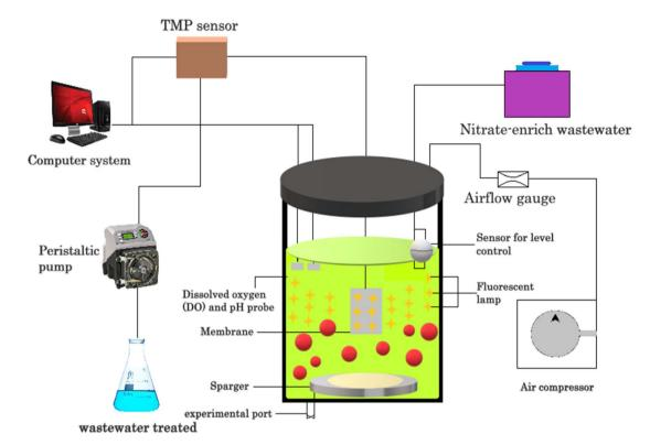
Fig. 6 Pollutant removal through algae membrane reactors.
