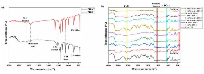
Fig. 3 FTIR of (a) ZIF-8 and ZIF-67, (b) pure PES and MMMs.
