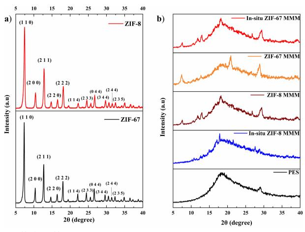
Fig. 2 XRD of (a) MOFs and (b) membranes.
