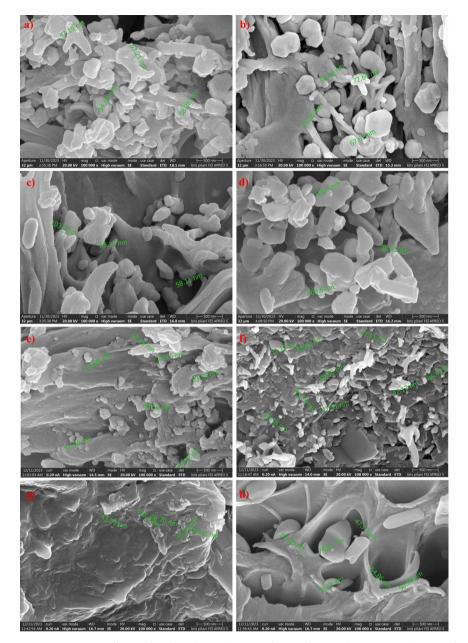
Fig. 4 FESEM images—cross-section view of (a and b) 1, 20 wt% ZIF-8 MMMs, (c and d) 1, 5 wt% in situ ZIF-8 MMMs, (e and f) 1, 20 wt% ZIF-67 MMMs, (g and h) 1, 5 wt% in situ ZIF-67 MMMs.
