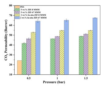
Fig. 5 Variation of CO<sub>2</sub> permeability of MMMs with the increase of pressure.
