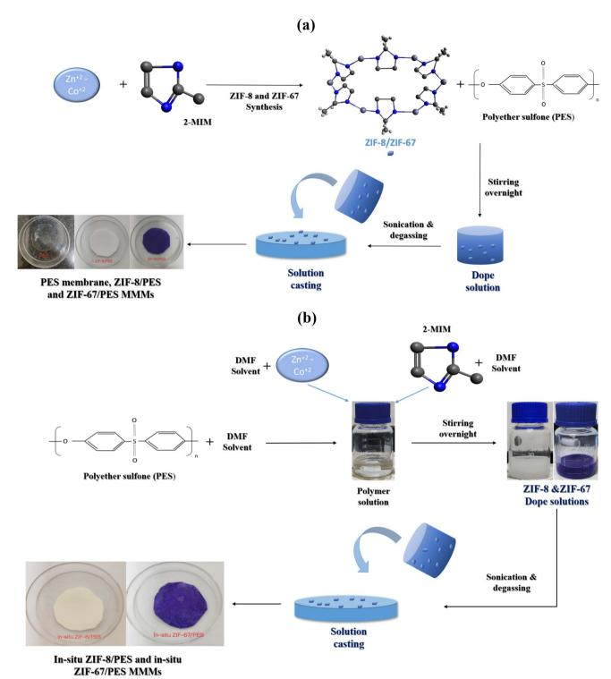
Fig. 1 Schematic for preparation of MMMs via (a) traditional method and (b) in situ method.
