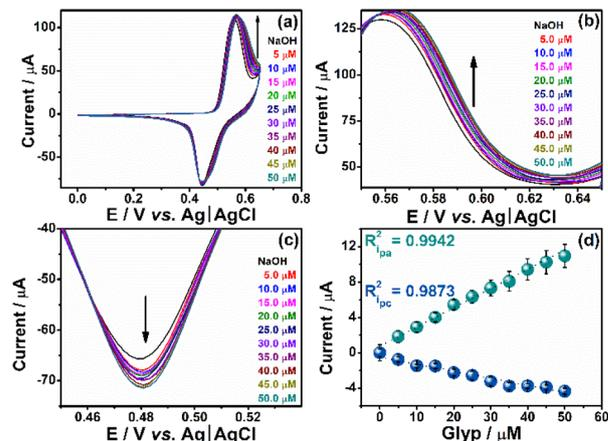
Fig. 5 (a) CV obtained for 10 additions, sequences of  $5.00 \mu\text{M}$  Glyp, (b) amplification of the analytical anodic region, (c) amplification of the cathodic analytical region, (d) linear range of the anodic and cathodic peaks respectively.
