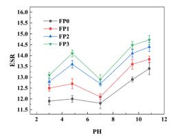
Fig. 5 pH responsiveness curve of Lys/P(AM-U-ChCl) composite hydrogel.
