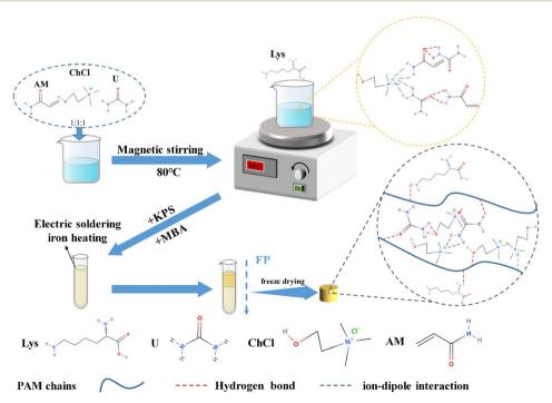
Fig. 2 Flow chart of Lys/P(AM-U-ChCl) composite hydrogel preparation.
