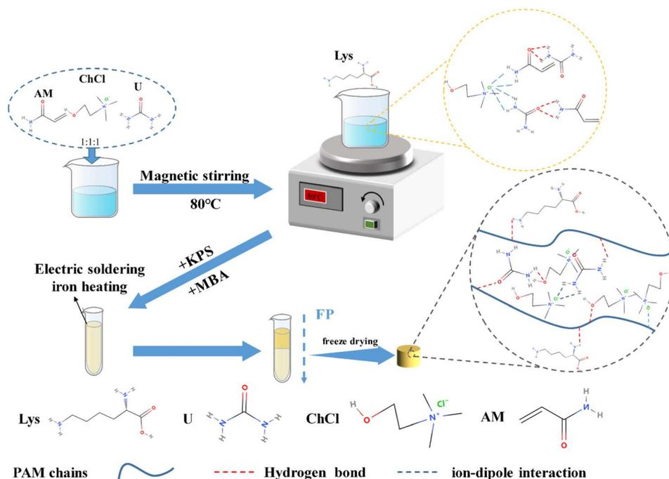
Fig. 2 Flow chart of Lys/P(AM-U-ChCl) composite hydrogel preparation.
