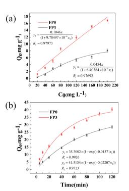
Fig. 9 (a) Langmuir adsorption profiles of Fe<sup>3+</sup> by FPO and FP3 hydrogels; (b) pseudo-primary adsorption profiles of Fe<sup>3+</sup> by FPO and FP3 hydrogels.
