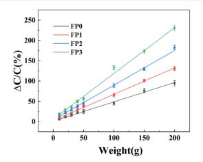
Fig. 7 Relative change in capacitance of Lys/P (AM-U-ChCl) hydrogel pressure sensor at different pressures.
