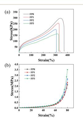
Fig. 6 (a) Hydrogel tensile performance test curve; (b) hydrogel compression performance test curve.
