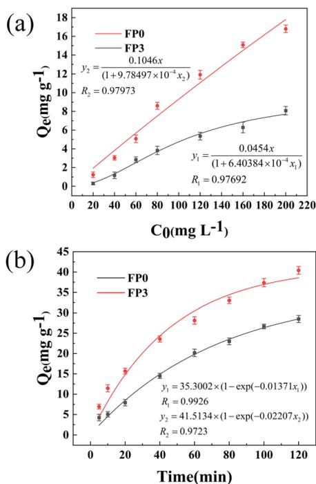
**Fig. 9** (a) Langmuir adsorption profiles of  $\text{Fe}^{3+}$  by FP0 and FP3 hydrogels; (b) pseudo-primary adsorption profiles of  $\text{Fe}^{3+}$  by FP0 and FP3 hydrogels.
