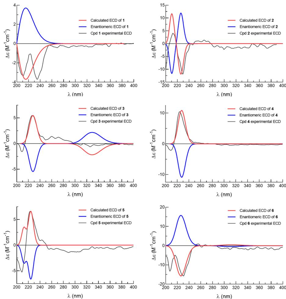
Fig. 4 Calculated and experimental ECD spectra of compounds 1–6.
