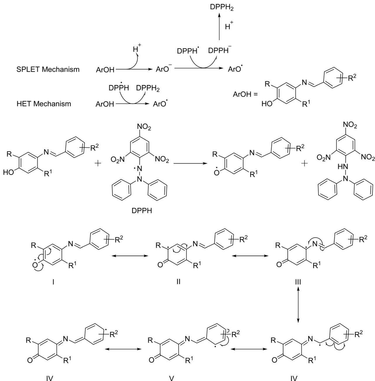
Fig. 5 Proposed mechanism of reaction of Schiff bases with DPPH.<sup>61</sup>
