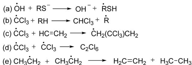
Fig. 2 Mechanism of reactions of free radicals.<sup>34</sup>
