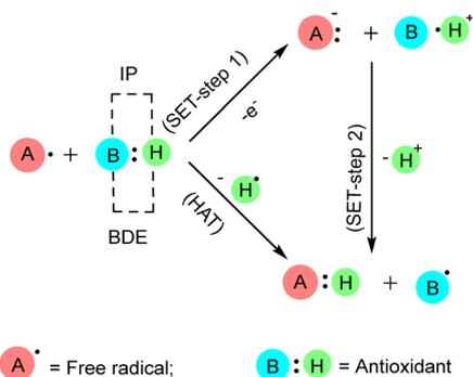
Fig. 4 Interaction of antioxidants with free radicals by SET and HAT. When measuring the antioxidant effect in SET mechanism, the IP (ionization potential) of the antioxidant is the most crucial energetic component. In the HAT mechanism, the BDE (bond dissociation enthalpy) of the antioxidant is crucial for assessing its effectiveness.<sup>38</sup>
