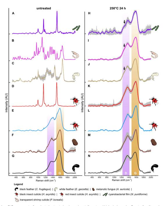
Fig. 1 Mean (n = 9) Raman spectra for selected untreated and experimentally matured biological samples. Spectra for all samples are shown in Fig. S5.† Grey area represents the standard deviation. Arrow indicates shoulder. White arrowhead on beetle cuticle indicates sampling location.
