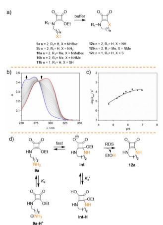
Fig. 4 (a) Structure of the squaramate esters 9a-10c and cyclic compounds 12a-12c. (b) Representative example of the UV changes observed for the cyclisation of 9a (30  $\mu$ M at 10 mM cacodylate buffer pH 5.7 at 37 °C). (c) Plot of the  $k_{\rm obs}$  obtained at pH range 4.5–7. The curve shows the fitting of the experimental data. (d) Proposed intramolecular addition–elimination mechanism for ester 9a to give cyclic squaramide 11a under mildly acidic conditions.
