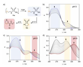
Fig. 5 (a) Synthetic scheme for synthesizing squaramate ester 11a, cyclothiosquaramide 11c, and the  $\alpha$ -keto carboxylate 13. UV changes observed for the hydrolysis of 11b after *in situ* reduction of 11a at (b) 30  $\mu$ M, 10 mM acetate buffer, pH 5, 37 °C, and (c) 30  $\mu$ M, 10 mM PBS buffer, pH 8, 37 °C. (d) UV changes of the degradation of the isolated 12c at 30  $\mu$ M, 10 mM PBS buffer, pH 8, 37 °C.
