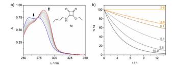
Fig. 2 (a) Changes observed in the UV spectra of 1a (blue trace) due to hydrolysis (30  $\mu$ M in 10 mM carbonate buffer, pH 10, 37 °C) as a representative example of the studied squaramate esters. Red trace represents the corresponding hydrolysed squaric acid. (b) Calculated disappearance of 1a (30  $\mu$ M, 37 °C) from the UV spectrum at different pH (10 mM carbonate buffer). From pH 3 to 8, no hydrolysis was observed after one week.
