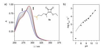
Fig. 3 (a) UV changes observed for the hydrolysis of ester 5a (30  $\mu$ M) at pH 9 (10 mM borate buffer) and 37 °C. (b) Data fitting to obtain  $k_1$  and  $k_{\mathrm{OH}}$ .
