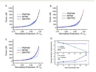
Fig. 3 Normalized F-E curves of PNIPAM and NPAM obtained in 0.1 M KSCN (A), 0.3 M KSCN (B), and 0.5 M KSCN (C) in comparison to the inherent F-E curve. (D) The energy difference to stretch PNIPAM and NPAM in solutions with different concentration in comparison to the inherent F-E curve.
