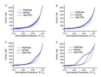
Fig. 2 Normalized experimental F-E curves of PNIPAM and NPAM in ultrapure water (A), 0.1 M KAc (B), 0.3 M KAc (C) and 0.5 M KAc (D) in comparison to the inherent F-E curve (red dotted line).
