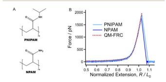
Fig. 1 (A) The chemical structures of PNIPAM and PNAM. (B) The typical normalized experimental force–extension (F–E) curves of PNIPAM and NPAM in DMSO (solid curves) compared to the theoretical inherent F–E curve of the C–C backbone.
