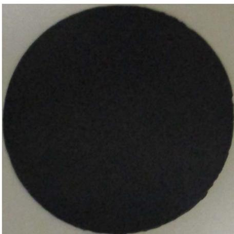
Fig. 5 A 4.7 cm diameter carbon nanotube buckypaper prepared via the electrolysis of CO<sub>2</sub> to form a carbanogel, grinding of 0.10 g of the product, dispersion with PVP in isopropanol, pressing, filtering, forming on the 0.2 μm pore nylon membrane, and lifting from the membrane.
