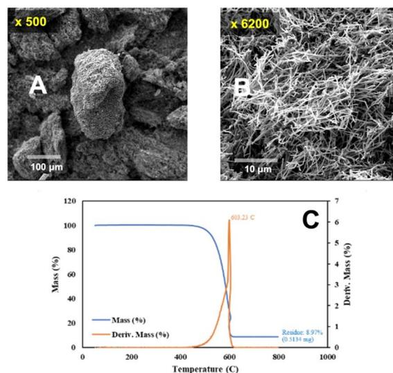
Fig. 4 (A) Medium and (B) higher magnification scanning electron microscopy images of the carbanogel particles composed of carbon nanotubes. (C) TGA of the carbanogel product, formed in 750  $^\circ\text{C}$   $\text{Li}_2\text{CO}_3$  at  $J = 0.09 \text{ A cm}^{-2}$ .
