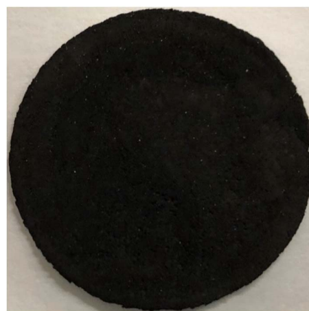
Fig. 3 A 4.7 cm diameter carbon nanotube buckypaper prepared via the electrolysis of CO 2 to form a carbanogel, grinding of the product, dispersion in isopropanol, pressing and filtering, and forming on a 0.2 μm pore nylon membrane.
