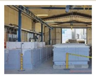
Fig. 2 The Genesis Device® kiln modules facilitate large-scale CO<sub>2</sub> molten carbonate electrolysis and was used in this study. Carbon Corp operates these modules in Calgary, Canada, for decarbonization.
