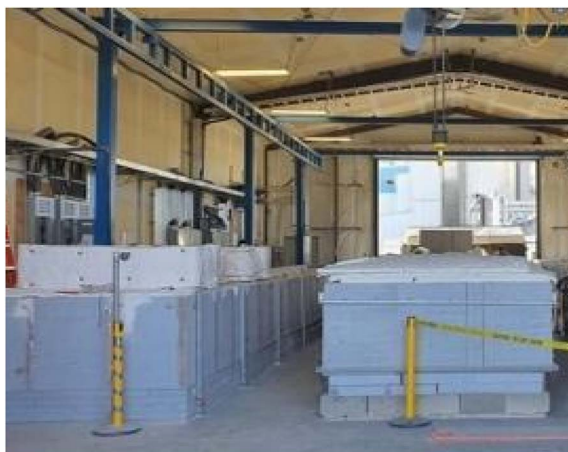
Fig. 2 The Genesis Device® kiln modules facilitate large-scale CO 2 molten carbonate electrolysis and was used in this study. Carbon Corp operates these modules in Calgary, Canada, for onsite decarbonization.
