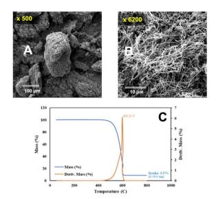
Fig. 4 (A) Medium and (B) higher magnification scanning electron microscopy images of the carbanogel particles composed of carbon nanotubes. (C) TGA of the carbanogel product, formed in 750 °C  $\text{Li}_2\text{CO}_3$  at  $J=0.09~\text{A}~\text{cm}^{-2}$ .
