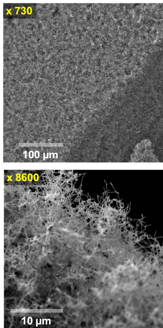
Fig. 1 Medium (top) and high (bottom) scanning electron microscopy images of the carbanogel particles comprised of carbon nanotubes formed at 770 °C Li<sub>2</sub>CO<sub>3</sub> at  $J = 0.4$  A cm<sup>-2</sup>.
