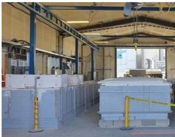
Fig. 2 The Genesis Device® kiln modules facilitate large-scale CO<sub>2</sub> molten carbonate electrolysis and was used in this study. Carbon Corp operates these modules in Calgary, Canada, for onsite decarbonization.
