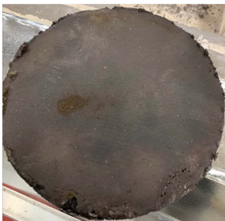
Fig. 6 A 35 cm diameter carbon nanotube buckypaper prepared via the electrolysis of CO 2 to form a carbanogel, and pressing of the carbanogel product while molten to separate residual carbanogel electrolyte from the graphene nanocarbon, carbon nanotube, and product.
