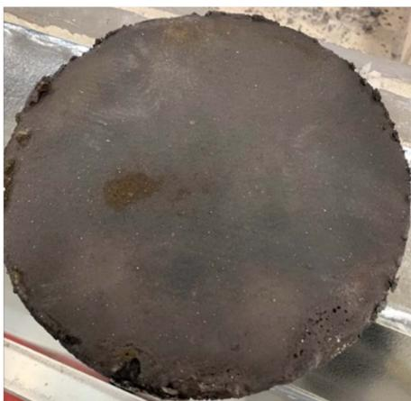
Fig. 6 A 35 cm diameter carbon nanotube buckypaper prepared via the electrolysis of CO<sub>2</sub> to form a carbanogel, and pressing of the carbanogel product while molten to separate residual carbanogel electrolyte from the graphene nanocarbon, carbon nanotube, and product.
