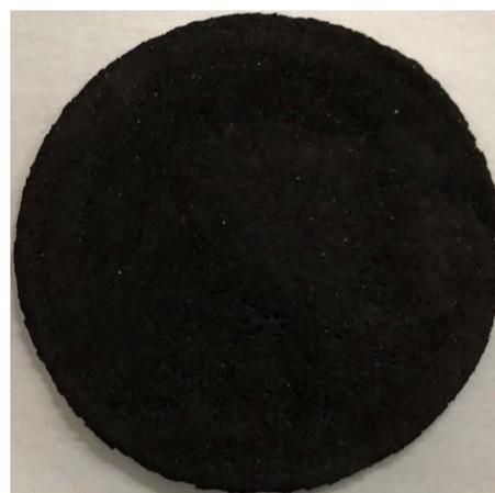
Fig. 3 A 4.7 cm diameter carbon nanotube buckypaper prepared via the electrolysis of CO<sub>2</sub> to form a carbanogel, grinding of the product, dispersion in isopropanol, pressing and filtering, and forming on a 0.2 μm pore nylon membrane.
