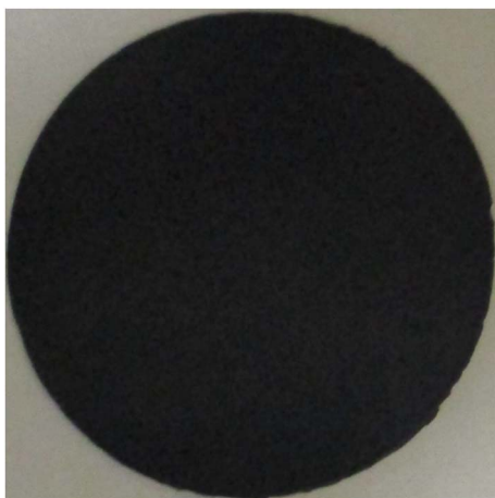
Fig. 5 A 4.7 cm diameter carbon nanotube buckypaper prepared via the electrolysis of CO 2 to form a carbanogel, grinding of 0.10 g of the product, dispersion with PVP in isopropanol, pressing, filtering, forming on the 0.2 μm pore nylon membrane, and lifting from the membrane.
