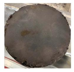
Fig. 6 A 35 cm diameter carbon nanotube buckypaper prepared via the electrolysis of  $CO_2$  to form a carbanogel, and pressing of the carbanogel product while molten to separate residual carbanogel electrolyte from the graphene nanocarbon, carbon nanotube, and product.
