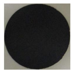
Fig. 5 A 4.7 cm diameter carbon nanotube buckypaper prepared  $\it via$  the electrolysis of  $CO_2$  to form a carbanogel, grinding of 0.10 g of the product, dispersion with PVP in isopropanol, pressing, filtering, forming on the 0.2  $\mu m$  pore nylon membrane, and lifting from the membrane.
