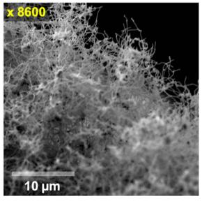
Fig. 1 Medium (top) and high (bottom) scanning electron microscopy images of the carbanogel particles comprised of carbon nanotubes formed at 770 °C  $\rm Li_2CO_3$  at  $J=0.4~\rm A~cm^{-2}$ .
