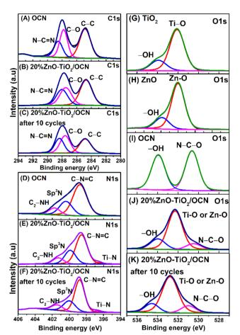
Fig. 2 High-resolution C 1s XPS spectra of TiO<sub>2</sub> (A), 20%ZnO-TiO<sub>2</sub>/ OCN (B), and 20%ZnO-TiO<sub>2</sub>/OCN after 5 cycles (C); high-resolution N 1s XPS spectra of OCN (D), 20%ZnO-TiO<sub>2</sub>/OCN (E) and 20%ZnO-TiO<sub>2</sub>/OCN after 10 cycles (F); high-resolution O 1s XPS spectra of TiO<sub>2</sub> (G), ZnO (H), OCN (I), 20%ZnO-TiO<sub>2</sub>/OCN (J) and 20%ZnO-TiO<sub>2</sub>/ OCN after 5 cycles (K).
