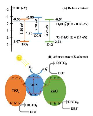
Fig. 9 Band structure of  $ZnO-TiO_2/OCN$  sample; (A) before contact and (B) after contact.
