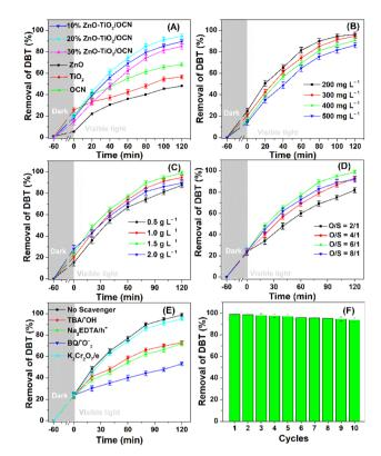
Fig. 8 (A) DBT conversion using ZnO,  $TiO_2$ , OCN and  $ZnO-TiO_2/OCN$  samples; DBT conversion using  $20\%ZnO-TiO_2/OCN$  at various initial DBT concentrations (B), catalyst dosage (C), O/S molar ratio (D), reactive radicals (E) and stability (F).
