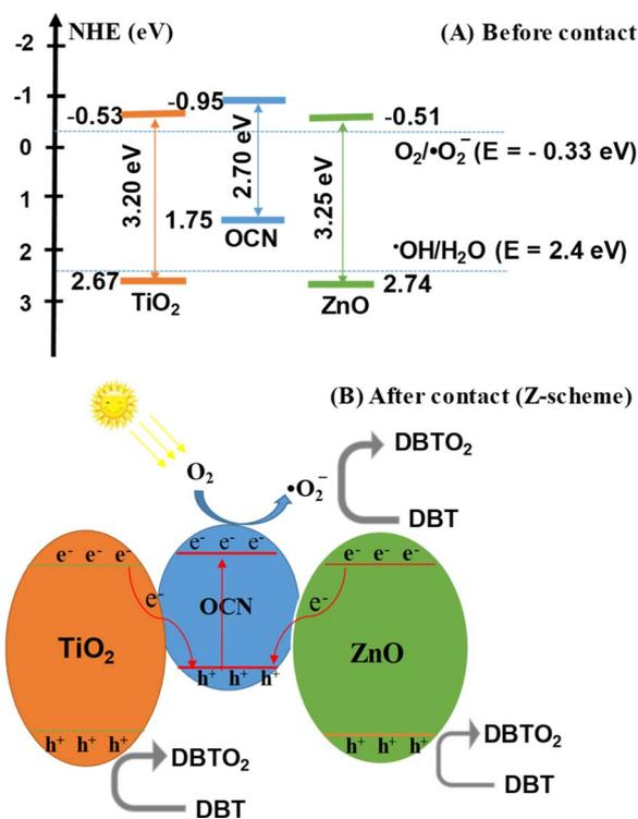
Fig. 9 Band structure of ZnO–TiO<sub>2</sub>/OCN sample; (A) before contact and (B) after contact.
