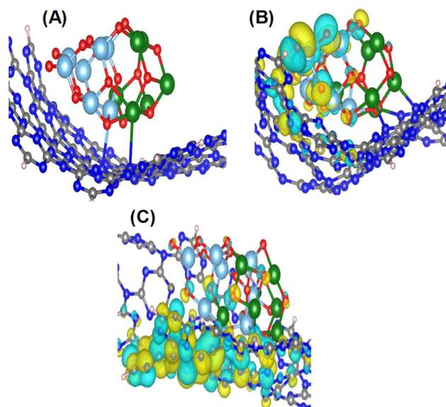
Fig. 10 Chemical bonding between (TiO<sub>2</sub>)<sub>7</sub>(ZnO)<sub>6</sub> with g-C<sub>3</sub>N<sub>4</sub> (A); images of HOMO (B) and LUMO (C) of ZnO-TiO<sub>2</sub>/OCN photocatalyst. Color codes: grey - C, blue - N, light blue - Ti, green - Zn, red - O.
