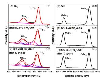
Fig. 3 High-resolution Ti 2p XPS spectra of TiO<sub>2</sub> (A), 20%ZnO-TiO<sub>2</sub>/ OCN (C) and 20%ZnO-TiO $_2$ /OCN after 5 cycles (E); high-resolution Zn 2p XPS spectra of ZnO (B), 20%ZnO-TiO<sub>2</sub>/OCN (D) and 20%ZnO-TiO<sub>2</sub>/OCN after 5 cycles (F).
