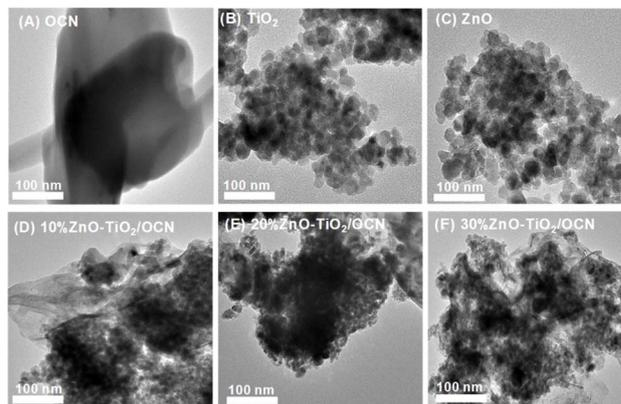
Fig. 5 TEM images of OCN, ZnO, TiO<sub>2</sub> and ZnO–TiO<sub>2</sub>/OCN samples.
