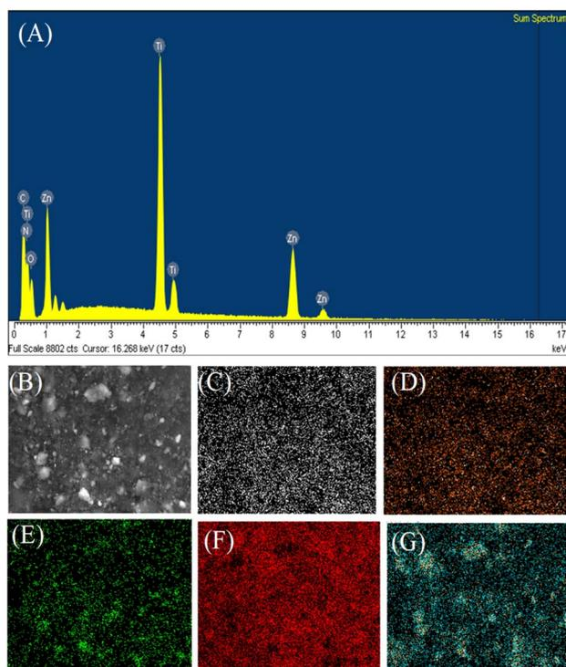
Fig. 4 EDS spectrum (A), EDS element layered image (B), EDS element mapping images of C (C), N (D), O (E), Ti (F) and Zn (G) of 20%ZnO–TiO<sub>2</sub>/OCN sample.
