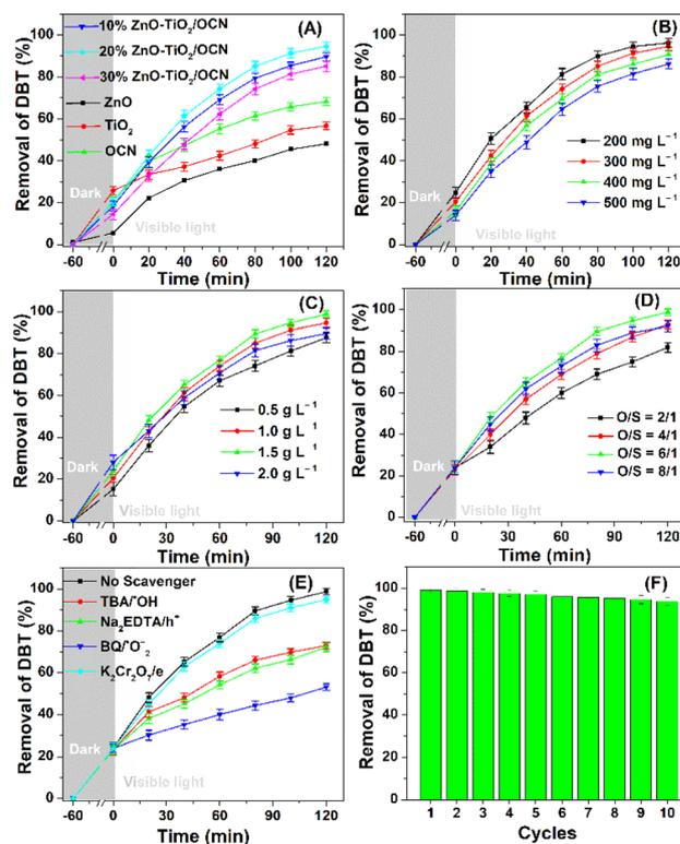
Fig. 8 (A) DBT conversion using ZnO, TiO<sub>2</sub>, OCN and ZnO–TiO<sub>2</sub>/OCN samples; DBT conversion using 20%ZnO–TiO<sub>2</sub>/OCN at various initial DBT concentrations (B), catalyst dosage (C), O/S molar ratio (D), reactive radicals (E) and stability (F).
