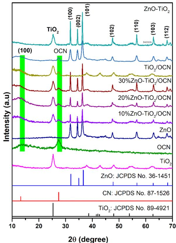
Fig. 1 XRD patterns of OCN, TiO<sub>2</sub>, ZnO, ZnO–TiO<sub>2</sub>, ZnO/OCN, TiO<sub>2</sub>/OCN and ZnO–TiO<sub>2</sub>/OCN samples.
