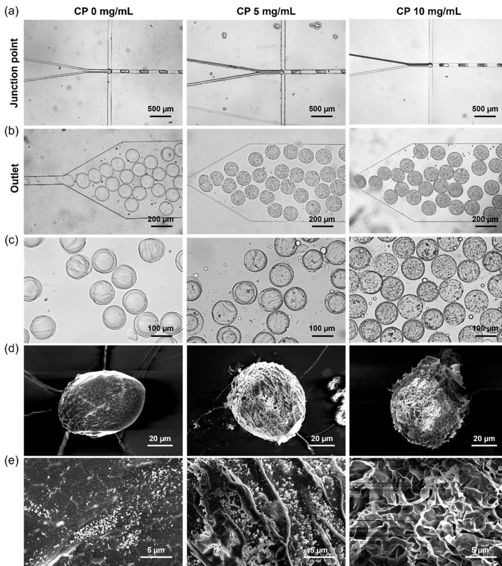
Fig. 3 Bright field images of microfluidic synthesis of Dex-MA microgels containing 0, 5 and 10 mg mL<sup>-1</sup> CP nanoparticles at (a) junction point and (b) outlet. (c) Bright field images of a purified Dex-MA microgel containing 0, 5 and 10 mg mL<sup>-1</sup> CP nanoparticles. SEM images of a freeze-dried Dex-MA microgel containing 0, 5 and 10 mg mL<sup>-1</sup> CP nanoparticles at (d) lower and (e) higher magnification.
