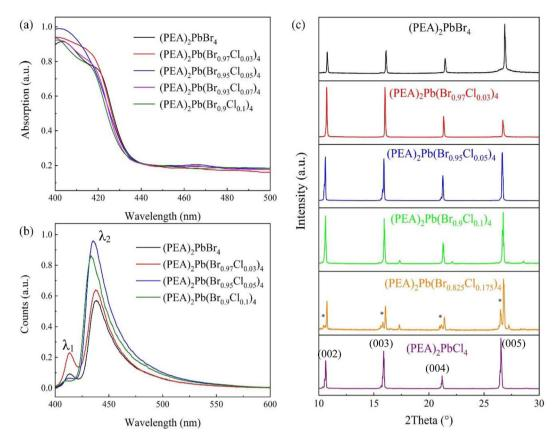
Fig. 2  $Cl^-$  doped (PEA)<sub>2</sub>PbBr<sub>4</sub>. (a) Absorption spectrum, (b) photoemission spectrum, and (c) powder XRD of (PEA)<sub>2</sub>PbBr<sub>4</sub>, (0, 3%, 5%, 10%, 17.5%, 100% doping concentration).
