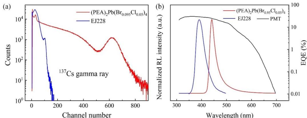
Fig. 5 (a) The light yield test using the gamma rays of  $^{137}\text{Cs}$  as the ray source, (b) RL spectra of  $(\text{PEA})_2\text{Pb}(\text{Br}_{0.95}\text{Cl}_{0.05})_4$  and EJ228 and external quantum efficiency curves of Hamamatsu CR173-Q1 photomultiplier tubes used.
