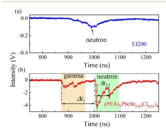
Fig. 7 Comparison of TOF test results of (PEA)<sub>2</sub>Pb(Br<sub>0.95</sub>Cl<sub>0.05</sub>)<sub>4</sub> crystal and plastic scintillator EJ228 in mixed field provided by DPF device.
