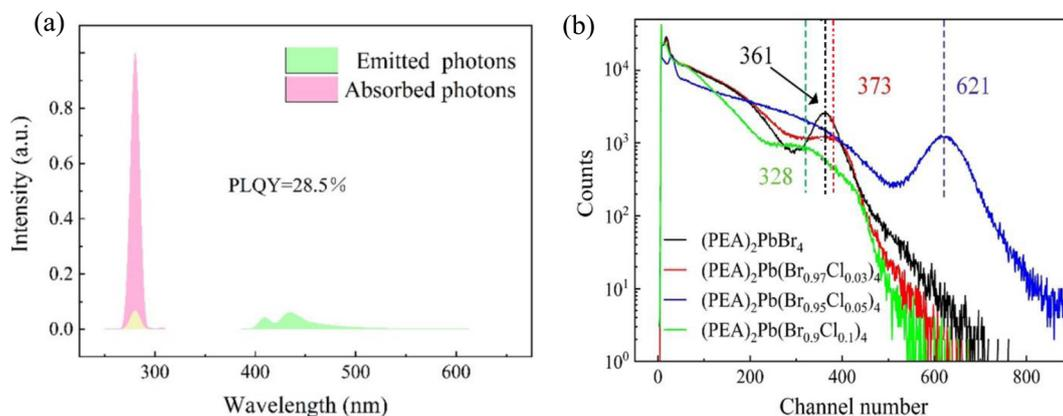
Fig. 3 (a) PLQY test results of 5% doping concentration crystal, (b) pulse amplitude spectra of  $(\text{PEA})_2\text{PbBr}_4$  crystals with different  $\text{Cl}^-$  doping concentrations ( $^{137}\text{Cs}$  source).
