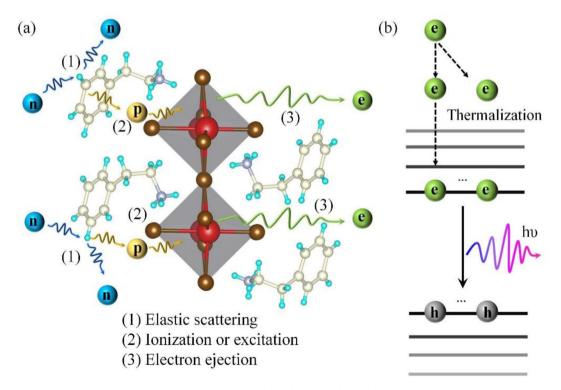
Fig. 6 Schematic diagram of the fast neutron detection principle of (PEA)<sub>2</sub>PbBr<sub>4</sub>, (a) and (b) were described from the perspective of space and energy band respectively.
