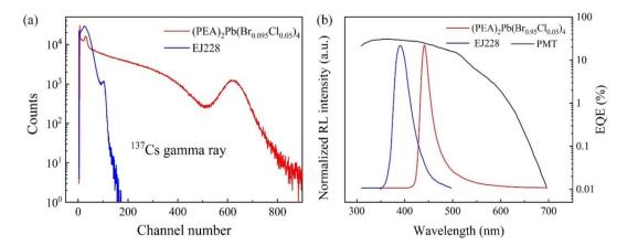
Fig. 5 (a) The light yield test using the gamma rays of  $^{137}$ Cs as the ray source, (b) RL spectra of (PEA)<sub>2</sub>Pb(Br<sub>0.95</sub>Cl<sub>0.05</sub>)<sub>4</sub> and EJ228 and external quantum efficiency curves of Hamamatsu CR173-Q1 photomultiplier tubes used.
