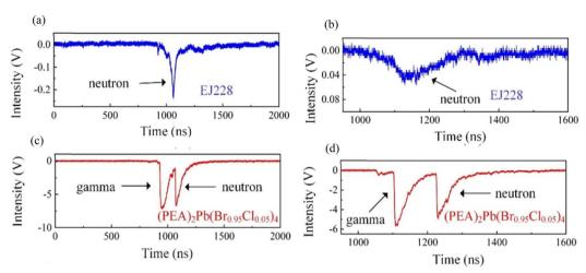
Fig. 8 Response test of  $(PEA)_2Pb(Br_{0.95}Cl_{0.05})_4$  crystal and plastic scintillator EJ228 in a DPF mixed field. (a) The response of plastic scintillator EJ228 from 0 to 2000 seconds, (b) the response of plastic scintillator EJ228 from 800 to 1600 seconds, (c) the response of  $(PEA)_2Pb(Br_{0.95}Cl_{0.05})_4$  crystal from 0 to 2000 seconds, (d) the response of  $(PEA)_2Pb(Br_{0.95}Cl_{0.05})_4$  crystal from 800 to 1600 seconds.
