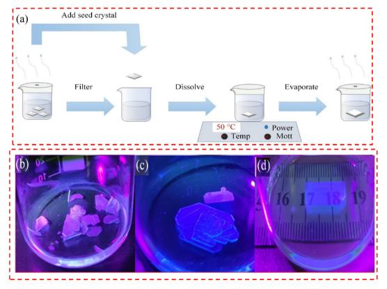
Fig. 1 (PEA)<sub>2</sub>PbBr<sub>4</sub> crystal growth process. (a) The flow chart of the entire single crystal growth process; (b) seedless induction growth; (c) seed induced dissolution growth without heating; (d) seed induced and heated dissolution growth.
