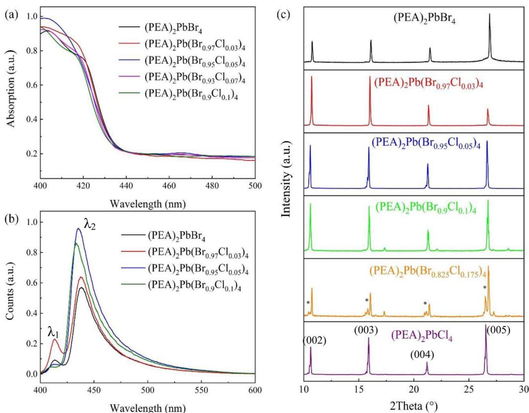
Fig. 2  $\text{Cl}^-$  doped  $(\text{PEA})_2\text{PbBr}_4$ . (a) Absorption spectrum, (b) photoemission spectrum, and (c) powder XRD of  $(\text{PEA})_2\text{PbBr}_4$ , (0, 3%, 5%, 10%, 17.5%, 100% doping concentration).
