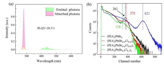
Fig. 3 (a) PLQY test results of 5% doping concentration crystal, (b) pulse amplitude spectra of  $(PEA)_2PbBr_4$  crystals with different  $Cl^-$  doping concentrations  $(^{137}Cs)$  source).
