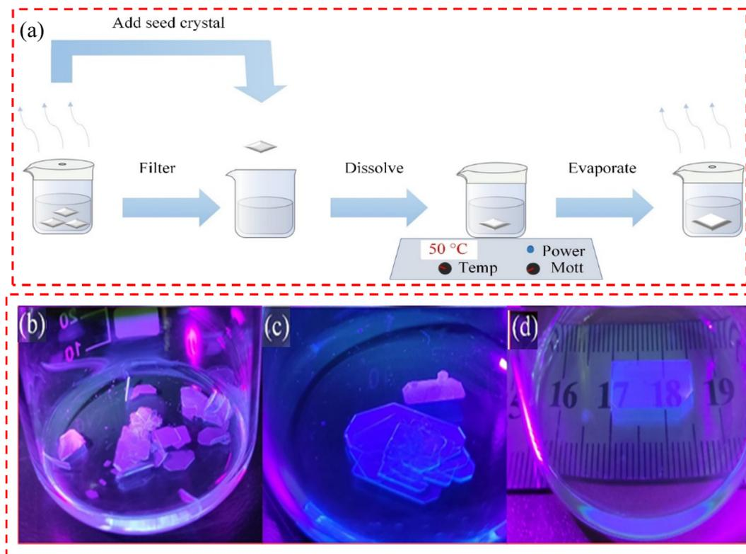
Fig. 1  $(\text{PEA})_2\text{PbBr}_4$  crystal growth process. (a) The flow chart of the entire single crystal growth process; (b) seedless induction growth; (c) seed induced dissolution growth without heating; (d) seed induced and heated dissolution growth.
