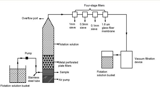
Fig. 1 Schematic diagram of microplastic extraction device.
