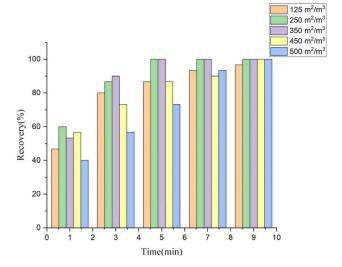
Fig. 3 Effect of metal perforated plate packing on microplastic
