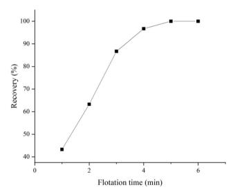
Fig. 5 Effect of flotation time on microplastic recovery.
