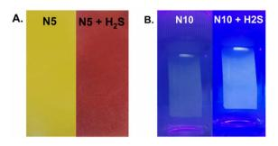
Fig. 11 Display of paper strip sensing of  $H_2S$  using (A) an N5-coated filter paper in the absence and presence of  $H_2S$ . (B) N10-coated paper strip under a UV lamp in the absence and presence of  $H_2S$ .
