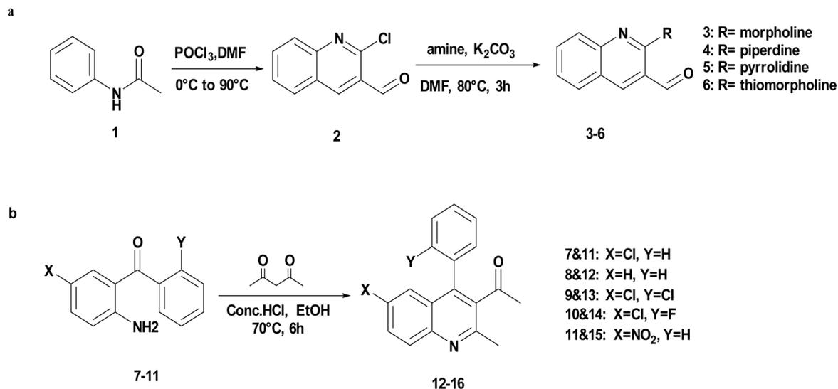
**Scheme 2** (a) Substrate scope of 2-(morpholine-piperidine-pyrrolidine-thiomorpholine) substituted quinoline-3-carbaldehyde (3–6). Reaction conditions: (2) (1 mmol), secondary amine (2 mmol), K<sub>2</sub>CO<sub>3</sub> (2 mmol). DMF (10 mL), 60 °C, 3 h (b) substrate scope of derivatives of quinoline (12–16). Reaction conditions: (7–11) (1 mmol), acetylacetone (4 mmol), EtOH (10 mL), and conc. HCl, 70 °C, 6 h.
