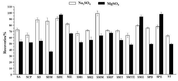
Fig. 4 Recoveries of the sulfonamides with different salt.
