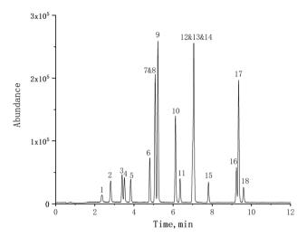
Fig. 2 The total ion flow chromatogram of blank forage grasses matrix spiked at 20  $\mu$ g L<sup>-1</sup>. (1) SA, (2) SD, (3) ST, (4) SPD, (5) SM1, (6) SM2, (7) SMTZ, (8) SMT, (9) SMP, (10) SMM, (11) SCP, (12) SDX-D<sub>3</sub>, (13) SDX, (14) SMZ, (15) SIZ, (16) SDM-D<sub>6</sub>, (17) SDM, (18) SPZ.
