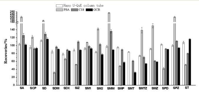
Recoveries of the sulfonamides with different purification sorbents
