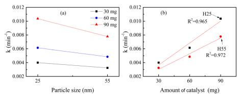
Fig. 7 Variation in reaction rate constant at room temperature with (a) particle size and (b) amount of catalyst.
