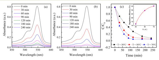
Fig. 4 Time-dependent spectral change in RB solutions catalyzed by 90 mg of H25 hematite nanoparticles at (a) 50 °C and (b) 70 °C; (c) variation in degradation with time at different steady temperatures; inset shows the variation in degradation efficiency with temperature 120 min after the irradiation of light.
