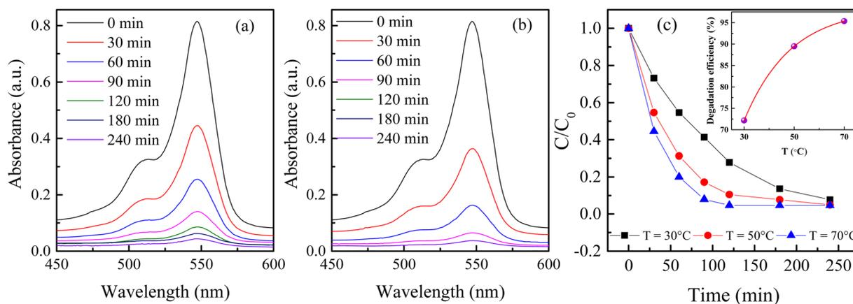
Fig. 4 Time-dependent spectral change in RB solutions catalyzed by 90 mg of H25 hematite nanoparticles at (a) 50 °C and (b) 70 °C; (c) variation in degradation with time at different steady temperatures; inset shows the variation in degradation efficiency with temperature 120 min after the irradiation of light.
