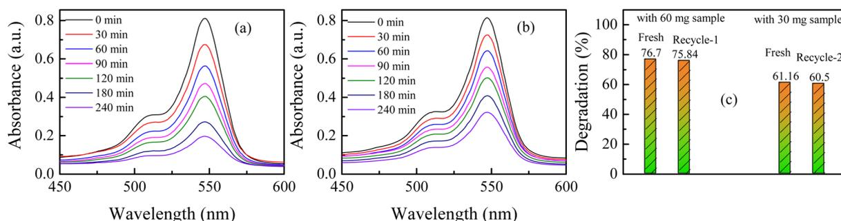
Fig. 10 Time-dependent spectral change in RB solution with H25 at room temperature: (a) recycle-1, (b) recycle-2; (c) comparison of degradation efficiency for recycle-1 and recycle-2 with fresh catalyst.
