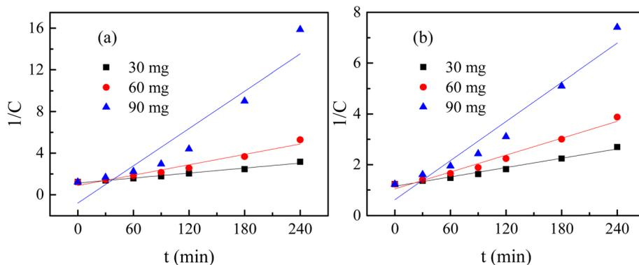
Fig. 6  $\frac{1}{C}$  vs.  $t$  plots for different amounts of catalyst at room temperature: (a) H25 and (b) H55.
