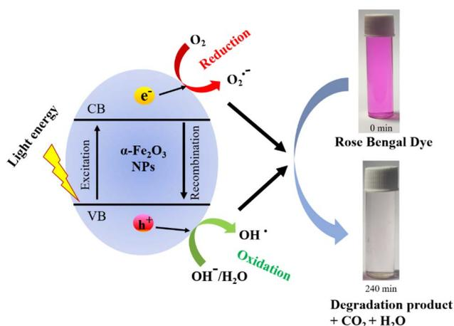
Scheme 2 Mechanism of rose bengal dye degradation.
