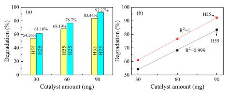
Fig. 3 (a) Variation in degradation efficiency with catalyst size and amount at room temperature. (b) Nature of variation in degradation of RB solution for H25 and H55 with catalyst amount at room temperature.
