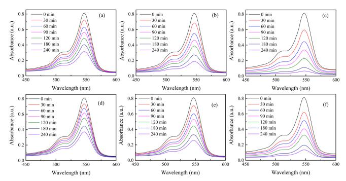
Fig. 1 Room temperature time-dependent spectral change in RB solution with (a) 30 mg, (b) 60 mg, and (c) 90 mg of H25 as the catalyst and (d) 30 mg, (e) 60 mg, and (f) 90 mg of H55 as the catalyst.
