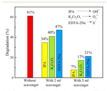
Fig. 9 Scavenger activity observed for photodegradation of RB with 30 mg of H25 catalyst at room temperature.
