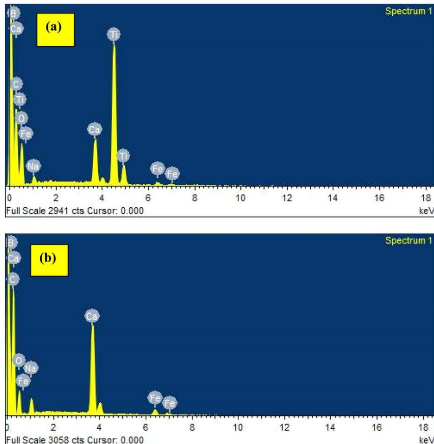
Fig. 5 (a) Elemental composition of the developed TiB/MWCNTs and (b) elemental composition of the developed B<sub>2</sub>O<sub>3</sub>/MWCNTs.
