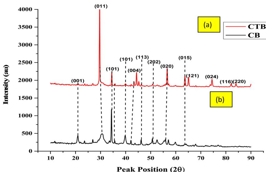
Fig. 6 XRD spectral of the developed (a) (CTB) TiB/MWCNTs and (b) (CB) B<sub>2</sub>O<sub>3</sub>/MWCNTs nano-adsorbent.
