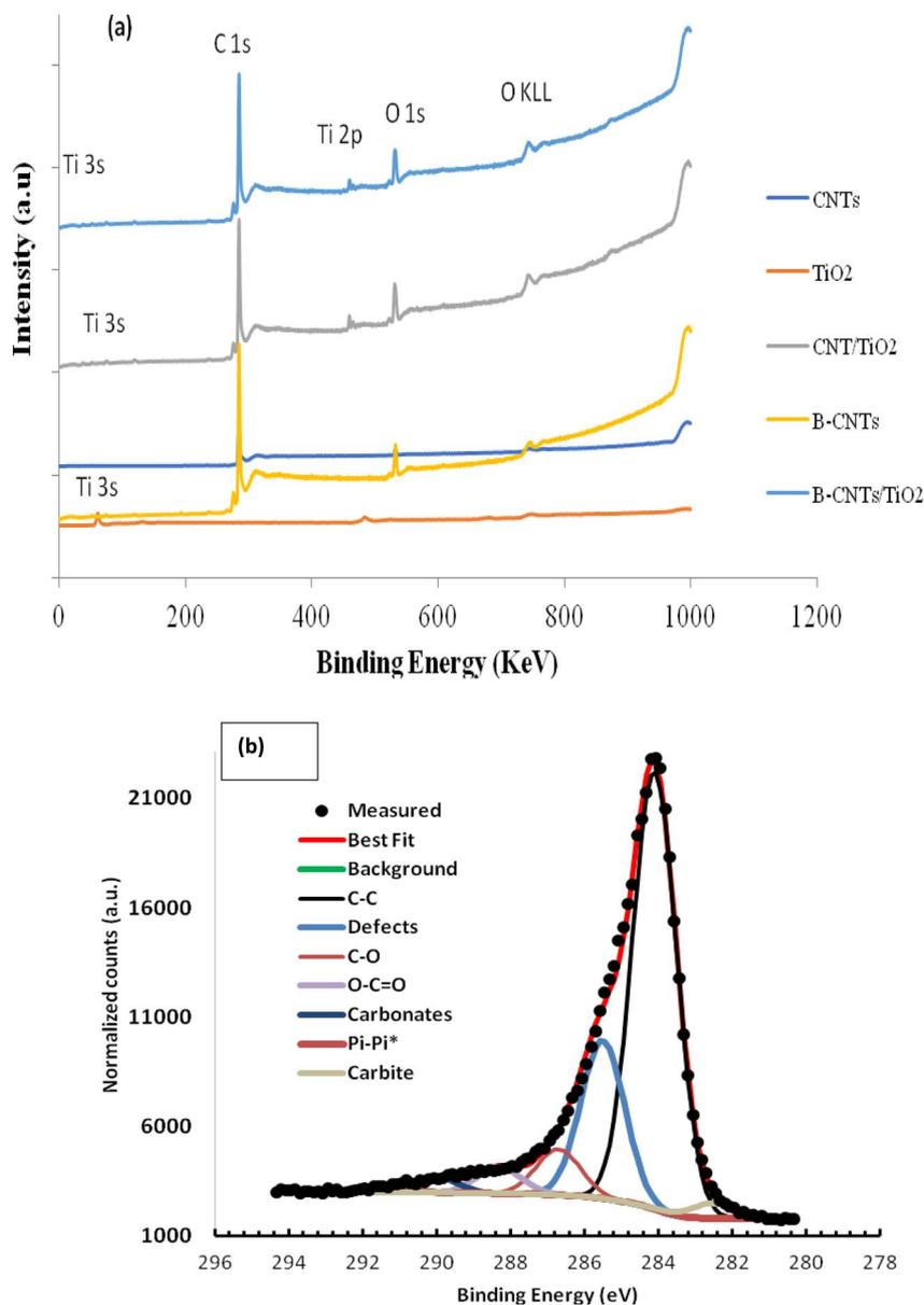
Fig. 8 (a) XPS survey of the developed nanoadsorbent (b) detailed XPS spectrum of TiB/MWCNTs and B<sub>2</sub>O<sub>3</sub>/MWCNTs nanoadsorbent.
