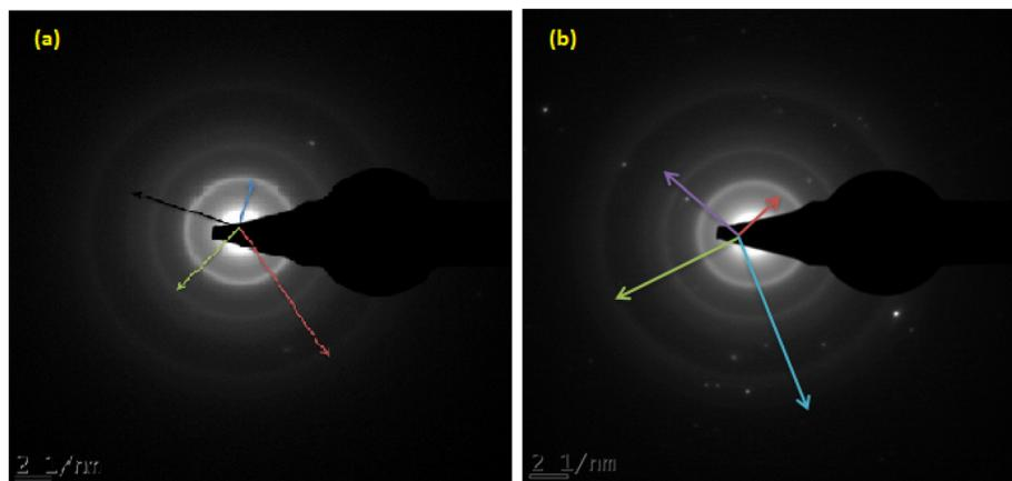
Fig. 7 SAED pattern of the developed (a) TiB/MWCNTs and (b) B<sub>2</sub>O<sub>3</sub>/MWCNTs nanoadsorbent.
