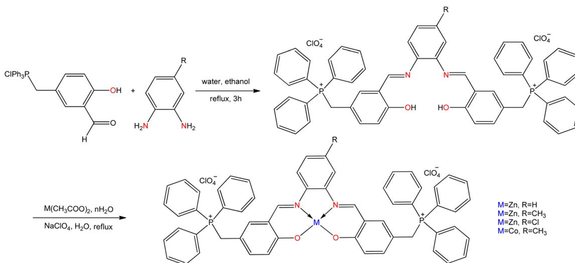
Fig. 16 Synthesis of Schiff base ligand and their metal complexes containing PPh<sub>3</sub><sup>+</sup> ion.
