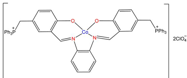
Fig. 25 The structure of the water-soluble cobalt(II) SB complex containing PPh<sub>3</sub> group.
