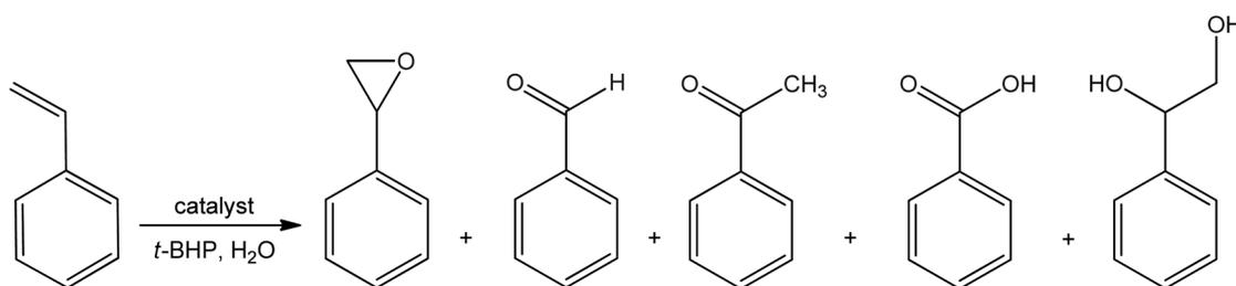
Fig. 5 Catalytic oxidation of styrene by oxovanadium(V) complexes.
