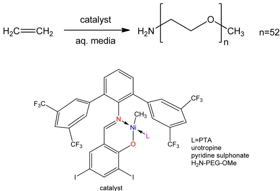
Fig. 1 Catalytic olefin polymerization by water-soluble Ni(II)-methyl complex.
