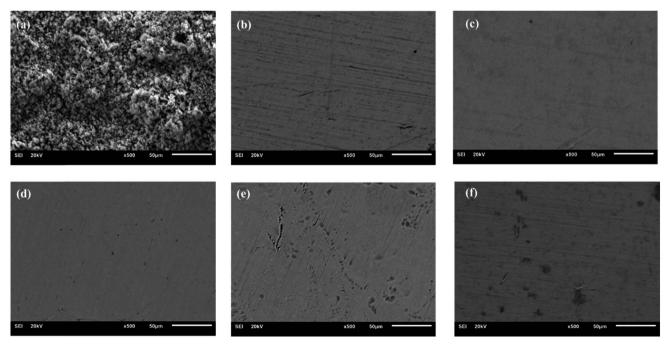
Fig. 5 The SEM of steel disks after corrosion test: (a) coating-free, (b) CMSCG (1:2), (c) CMSCG (1:1), (d) CMSCG (2:1), (e) MSCG, (f) CSCG.
