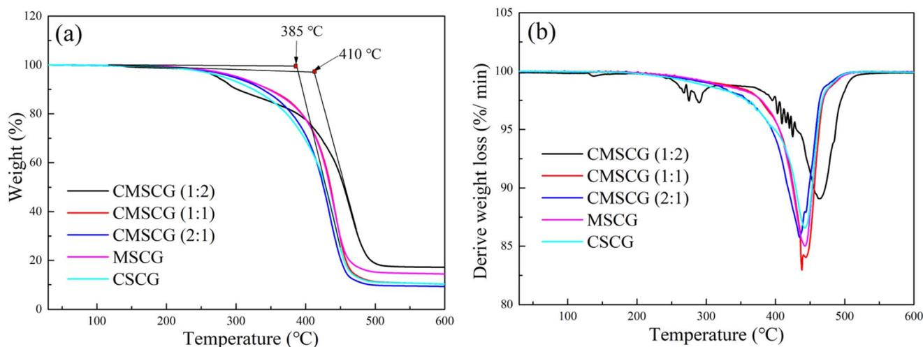
**Fig. 4** The TGA and DTG curves of grease, (a) TGA, (b) DTG.
