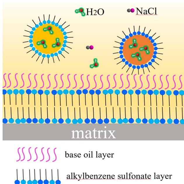
Fig. 8 The corrosion resistance mechanism of as-prepared grease.
