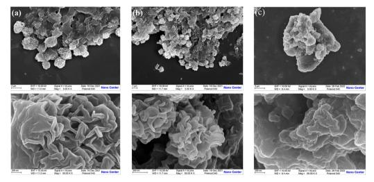
Fig. 3 The SEM images of thickener with different components, (a) CMSCG (1:1), (b) MSCG, (c) CSCG.
