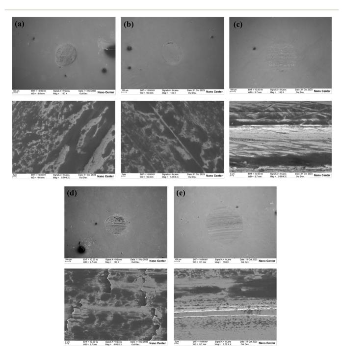
Fig. 11 The surface morphology of the wear scar at 392 N, (a) CMSCG (1:2), (b) CMSCG (1:1), (c) CMSCG (2:1), (d) MSCG, (e) CSCG.
