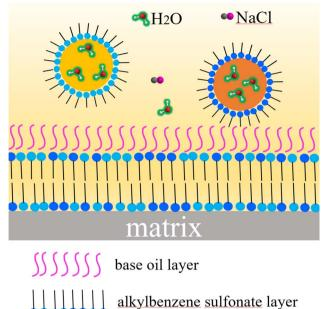
Fig. 8 The corrosion resistance mechanism of as-prepared grease.
