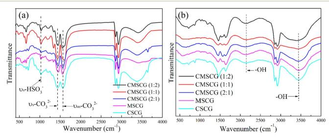
The FTIR of as-prepared grease before and after salt spray test, (a) before salt spray test, (b) after salt spray test
