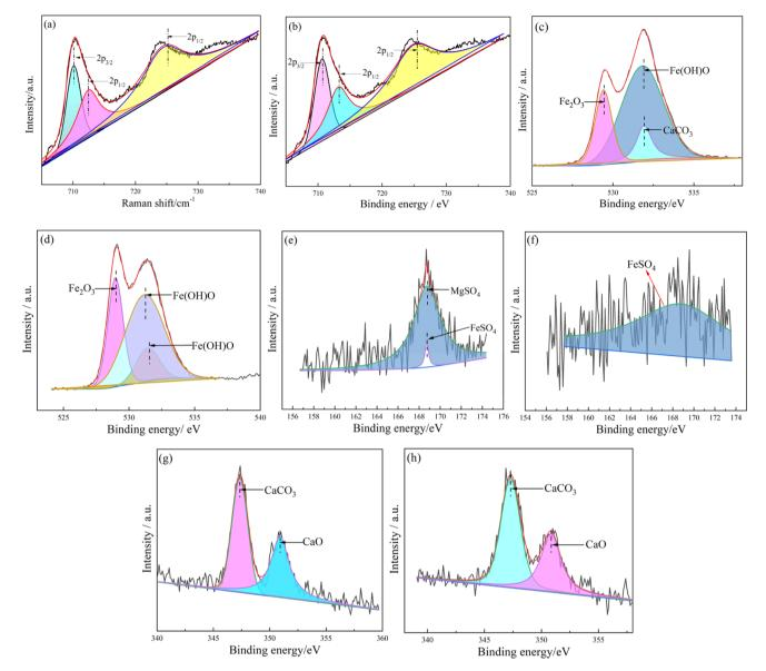
Fig. 13 The deconvoluted XPS spectra of wear scar lubricated by MSCG and CSCG, (a and b) Fe 2p, (c and d) O 1s, (e and f) S 2p, (g and h) Ca 2p.
