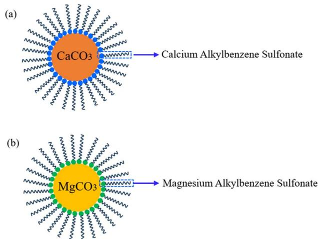
Fig. 1 The structural diagram of T106D and T107, (a) T106D, (b) T107.
