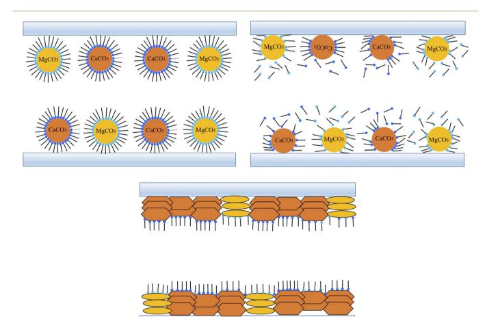
Fig. 14 The evolution of the overbased sulfonates during the friction.
