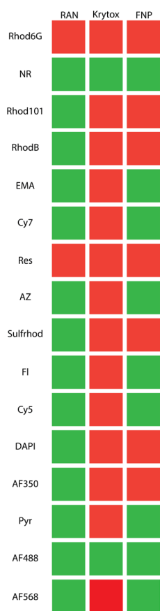
Fig. 3 Comparison of dye partitioning from aqueous phase into oil phase (HFE 7500) containing RAN, Krytox or FNPs. Samples were compared with one-sided t -test assuming variance and normal distribution. Colours were given according to p -values green for p -value > 0.01 red for p -value < 0.01. Dyes were sorted based on the distribution coefficients in DPBS.
