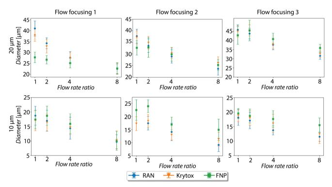
Fig. 9 Droplet size in function of the flow rate ratio (flow rate of the oil phase/flow rate of the aqueous phase) for three different flow focusing designs with 2% Krytox, 2% RAN and FNPs
