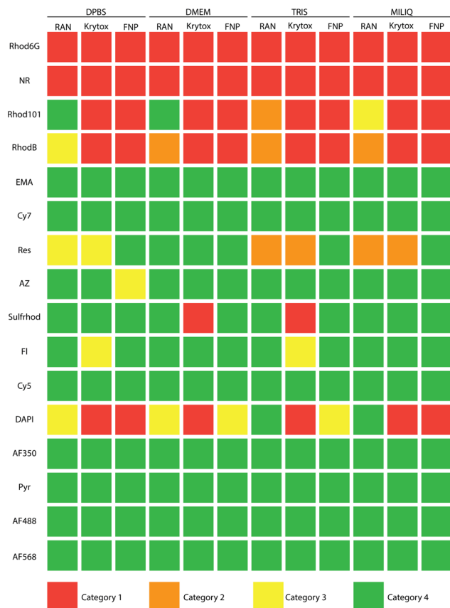
Fig. 5 Colour coded overview of leakage between droplet. Dyes are sorted based on distribution coefficient in DPBS (at the top the most hydrophobic dyes and at the bottom the more hydrophilic ones).
