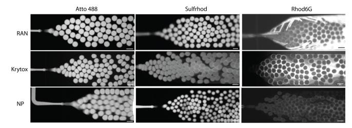
Fig. 6 On chip droplet production for three different dyes and three different surfactant, imaged with Nikon Ti2 (100 μM scale bar)
