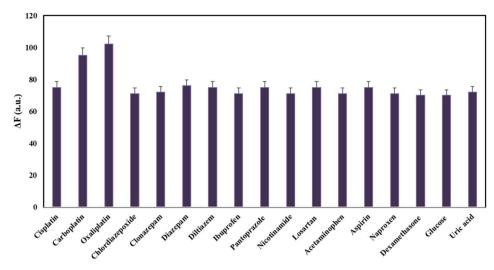
Fig. 4 Study of the method selectivity under optimal conditions in the presence of some possible interfering co-administrated drugs with concentrations of  $16.0 \text{ ng mL}^{-1}$ .
