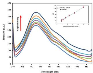
Fig. 3 Fluorescence intensity of GQDs/PVA hydrogel nanocomposite in the absence and presence of cisplatin in the range of 4.3 to 25.0 ng mL<sup>-1</sup>. Inset: Calibration curve obtained for cisplatin in urine.
