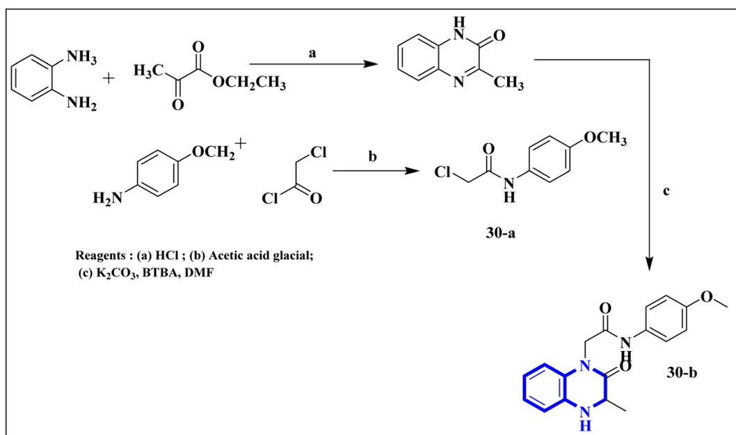
Fig. 20 Synthetic route *N*-(4-methoxyphenyl)-2-(3-methyl-2-oxo-3,4-dihydroquinoxalin-1(2*H*)-yl)acetamide, compound 30-b.<sup>30</sup>
