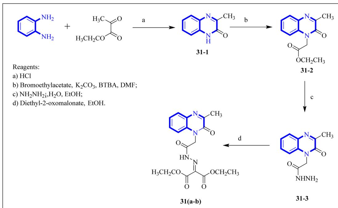
Fig. 21 Synthetic route 2-(2-(2-(3-methyl-2-oxoquinoxalin-1(2*H*)-yl)acetyl)hydrazono)malonate, **31(a-b)**.<sup>31</sup>
