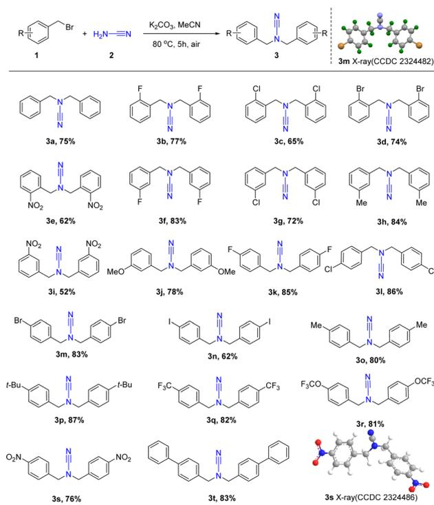
**Scheme 2** The substrate scope of the *N,N*-functionalized cyanamide **3**. Conditions of reaction: **1a** (0.44 mmol), **2a** (0.20 mmol), K<sub>2</sub>CO<sub>3</sub> (0.60 mmol) in MeCN (5 mL) stirred for 5 h at 80 °C at air, isolated yields.
