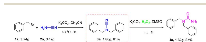
Scheme 4 Gram-scale synthesis of 4a . Conditions of reaction: 1a (22.0 mmol), 2a (10.0 mmol), K_2CO_3 (30.0 mmol) in MeCN (25 mL) stirred for 5 h at 80 °C under air atmosphere, isolated yields; 3a (8.1 mmol), H_2O_2 (9.7 mmol), K_2CO_3 (8.1 mmol) in DMSO (15 mL) stirred for 4 h at r.t. under air, isolated yields.
