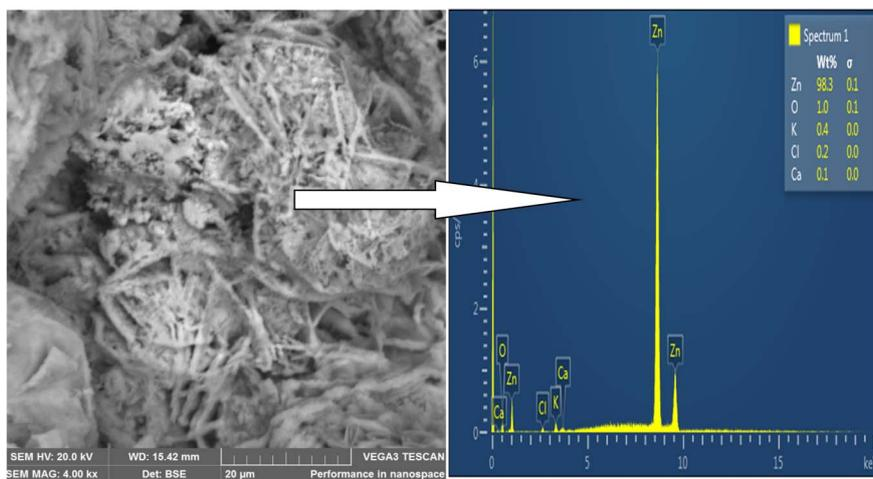
Fig. 6 SEM image of Zn-8% ESAP.
