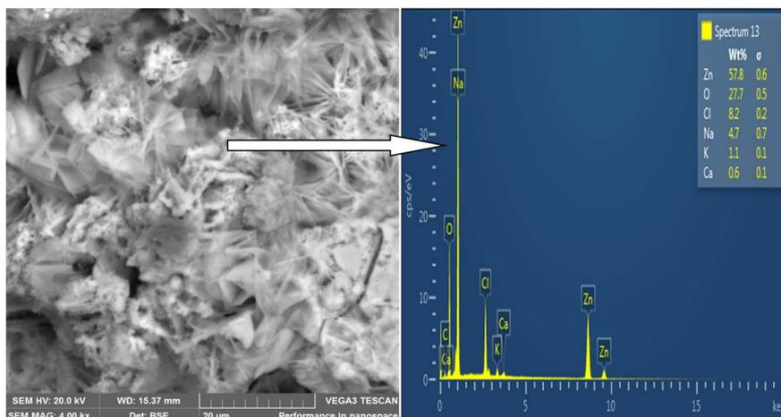
Fig. 7 SEM image of Zn-8% ESAP + 2% starch.
