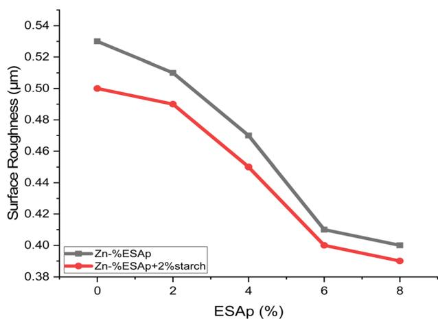
Fig. 2 Variation of surface roughness with %ESAp.
