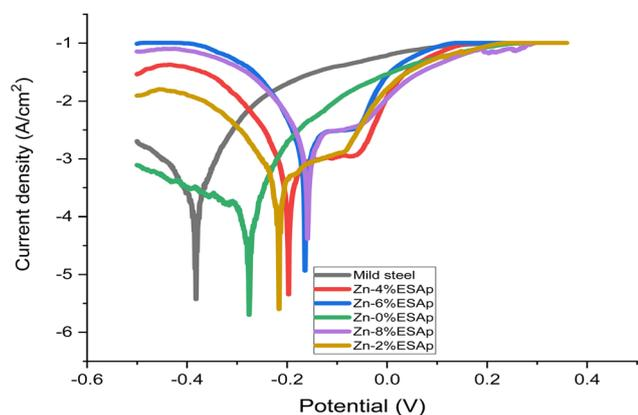
Fig. 10 Tafel extrapolation data of the Zn-ESAp samples.
