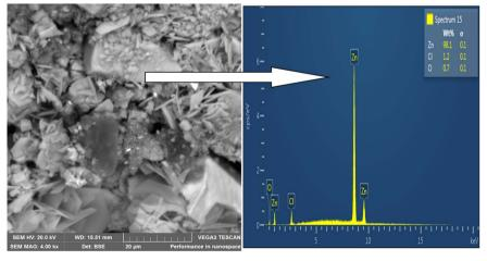
Fig. 5 SEM image of Zn-0% ESAp.
