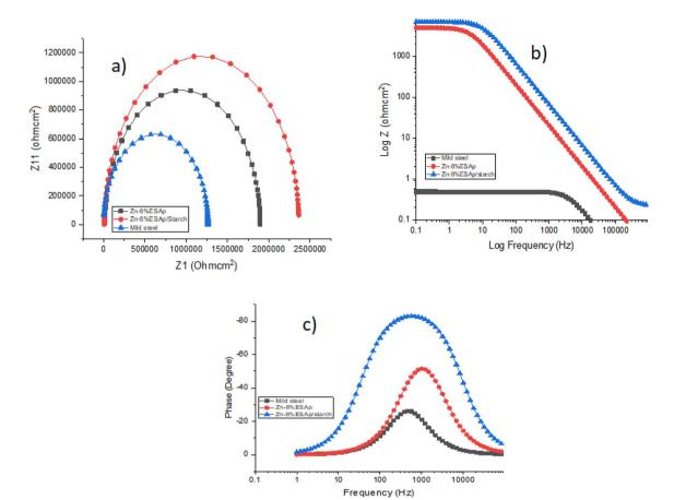
Fig. 12 (a) Nyquist plots (b) Bode impedance plots (c) Bode phase angle plots.
