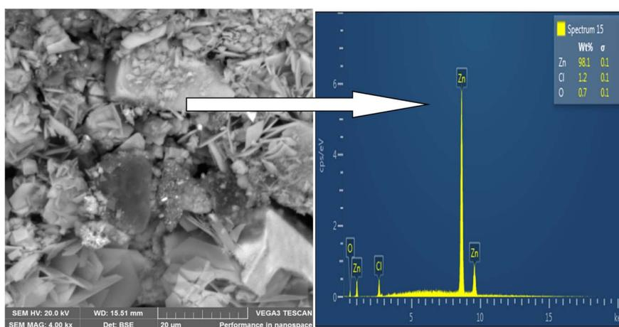
Fig. 5 SEM image of Zn-0% ESAP.
