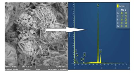
Fig. 6 SEM image of Zn-8% ESAp.
