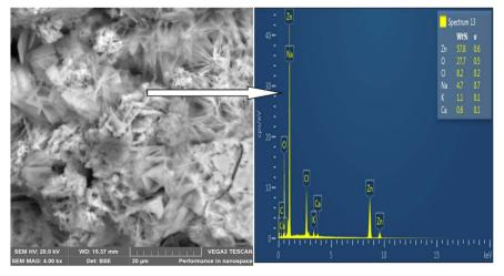
Fig. 7 SEM image of Zn-8% ESAp + 2% starch.
