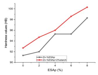
Fig. 15 Variation of hardness values with %ESAp.
