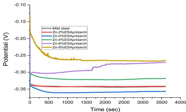
Fig. 9 OCP of the Zn-ESAp + 2% starch samples.
