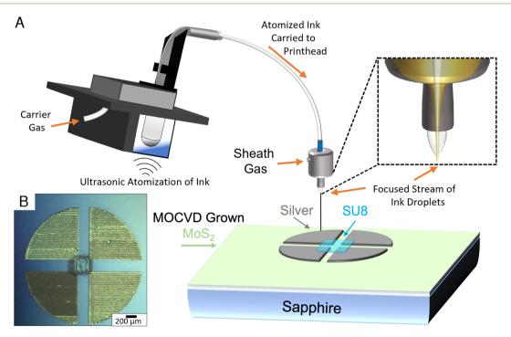
Fig. 4 (A) Cartoon schematic illustrating the aerosol jet printing process and the deposition of a silver van der Pauw 4-point device with a printed SU-8 passivation region on MOCVD MoS<sub>2</sub>. (B) Optical microscope image of the AJ-printed device after curing of SU-8 and removal of excess TMD material.
