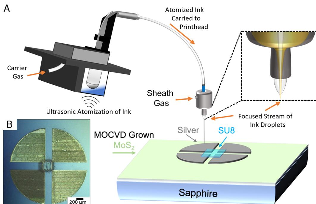
Fig. 4 (A) Cartoon schematic illustrating the aerosol jet printing process and the deposition of a silver van der Pauw 4-point device with a printed SU-8 passivation region on MOCVD MoS<sub>2</sub>. (B) Optical microscope image of the AJ-printed device after curing of SU-8 and removal of excess TMD material.
