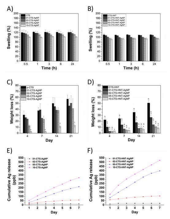
Fig. 6 (A and B) Water absorption capacity (swelling percentage) of the sponges, (C and D) degradation rate of the sponges incubated in PBSlysozyme solution, and (E and F) cumulative silver release from the sponges immersed in PBS.
