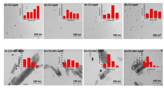
Fig. 2 Representative tem micrographs of the synthesized CTS/AgNPs and CTS/HNT/AgNPs nanocomposites as colloidal suspensions.
