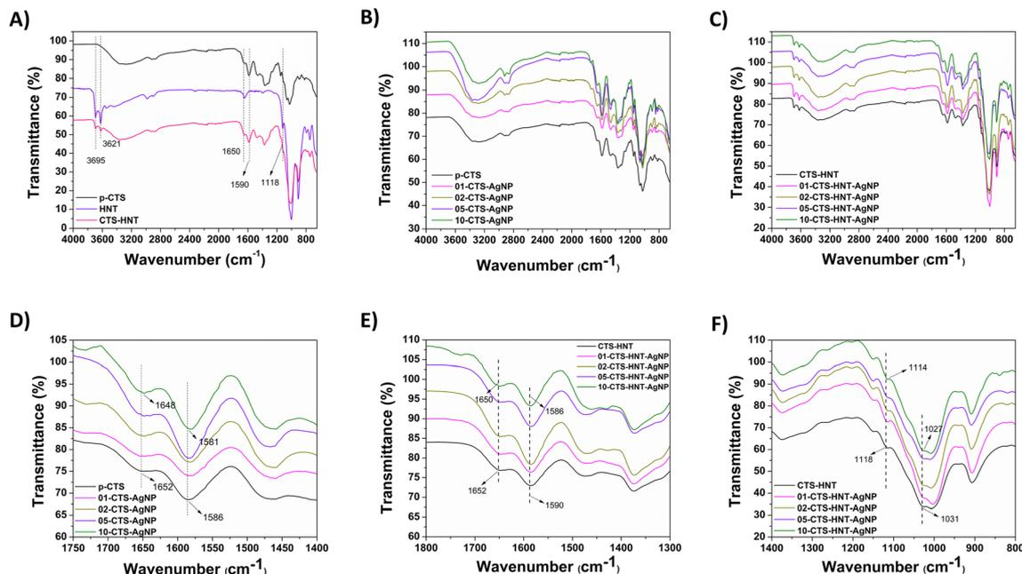
Fig. 5 FTIR spectra of (A) as received HNTs and p-CTS and CTS–HNT sponges, (B) p-CTS and CTS/AgNPs sponges, (C) CTS–HNT and CTS/HNT/AgNPs sponges. Magnification of the FTIR spectra exhibiting the (D) upshifting of the main cts bands occurring in the (D) CTS/AgNPs and (E) CTS/HNTs/AgNPs sponges. (F) Magnification of the FTIR spectra exhibiting the downshifting of the main hnts bands occurring in the CTS/HNTs/AgNPs sponges.
