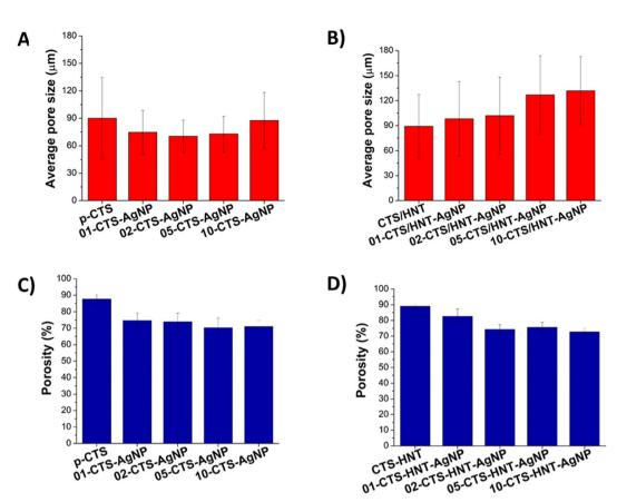
Fig. 4 (A and B) Pore size distribution and (C and D) porosity percentage of the CTS/AqNPs and CTS/HNT/AqNPs sponges.
