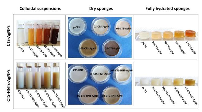
Fig. 1 Representative photographs of the macroscopic appearance of the synthesized CTS/AqNps and CTS/HNTs/AqNPs nanocomposites as colloidal suspensions, after the gelation process as sponges in their dry state, and after full hydration of the sponges.
