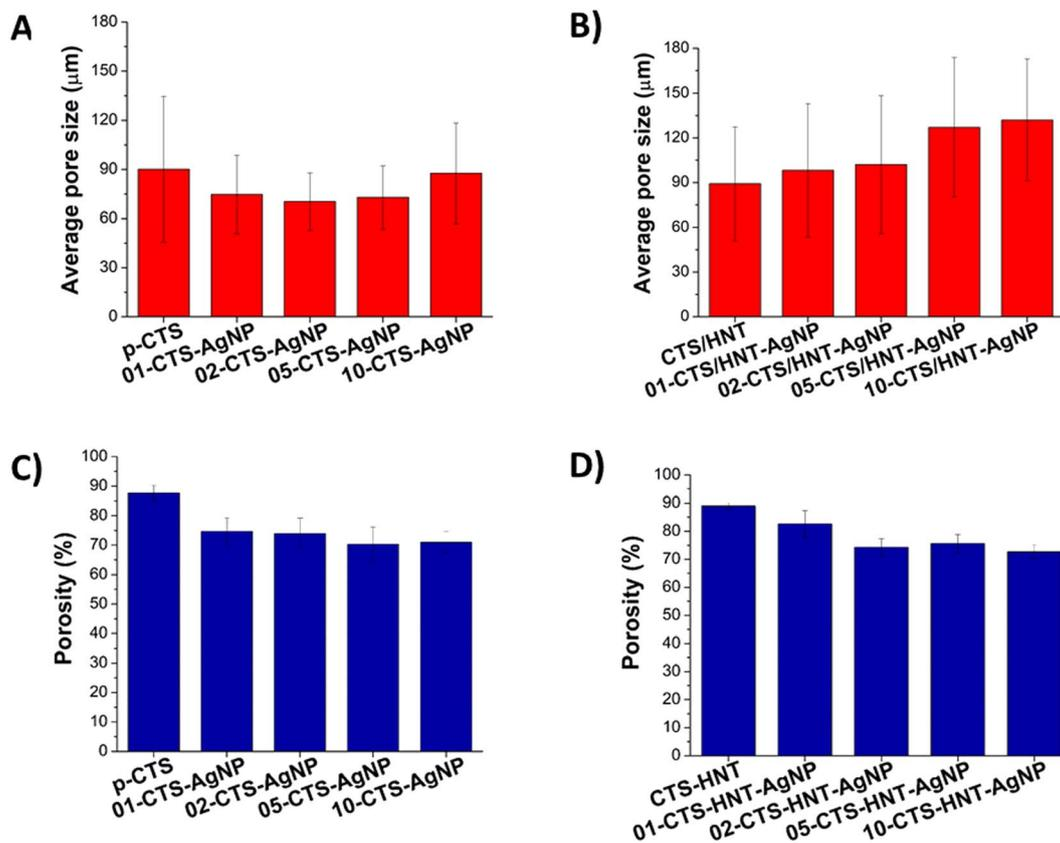
Fig. 4 (A and B) Pore size distribution and (C and D) porosity percentage of the CTS/AgNPs and CTS/HNT/AgNPs sponges.
