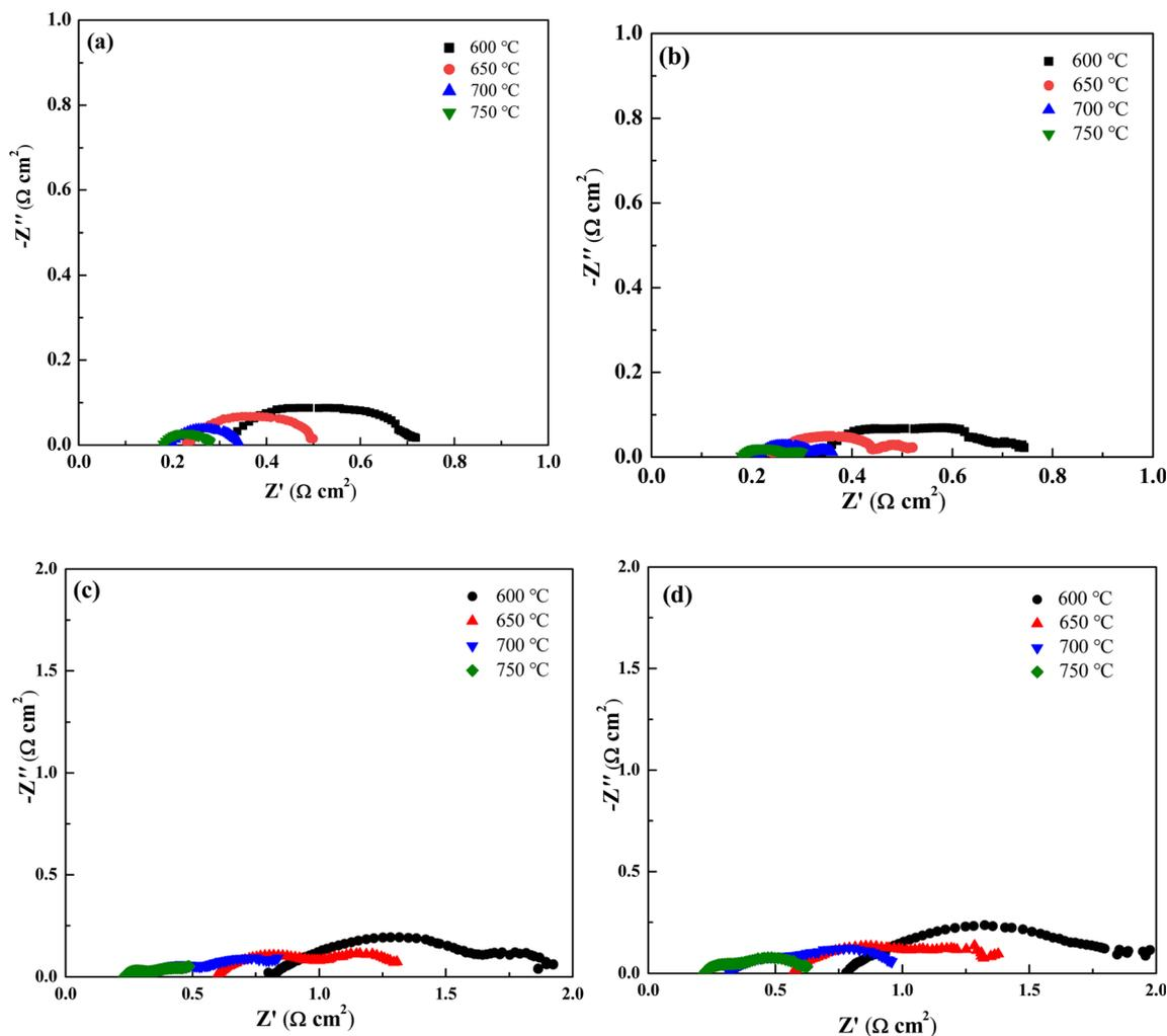
Fig. 4 The impedance spectra of cathode-impregnated (a) and full cell impregnated (b) MSCs under  $\text{H}_2$  atmosphere, and the impedance spectra of cathode-impregnated (c) and full cell impregnated (d) MSCs under  $\text{CH}_4$  atmosphere.
