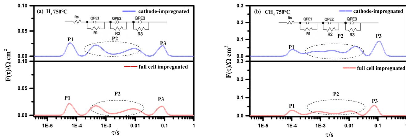
Fig. 5 DRT analysis of the two cells at 750 °C in an H<sub>2</sub> atmosphere (a) and a CH<sub>4</sub> atmosphere (b).
