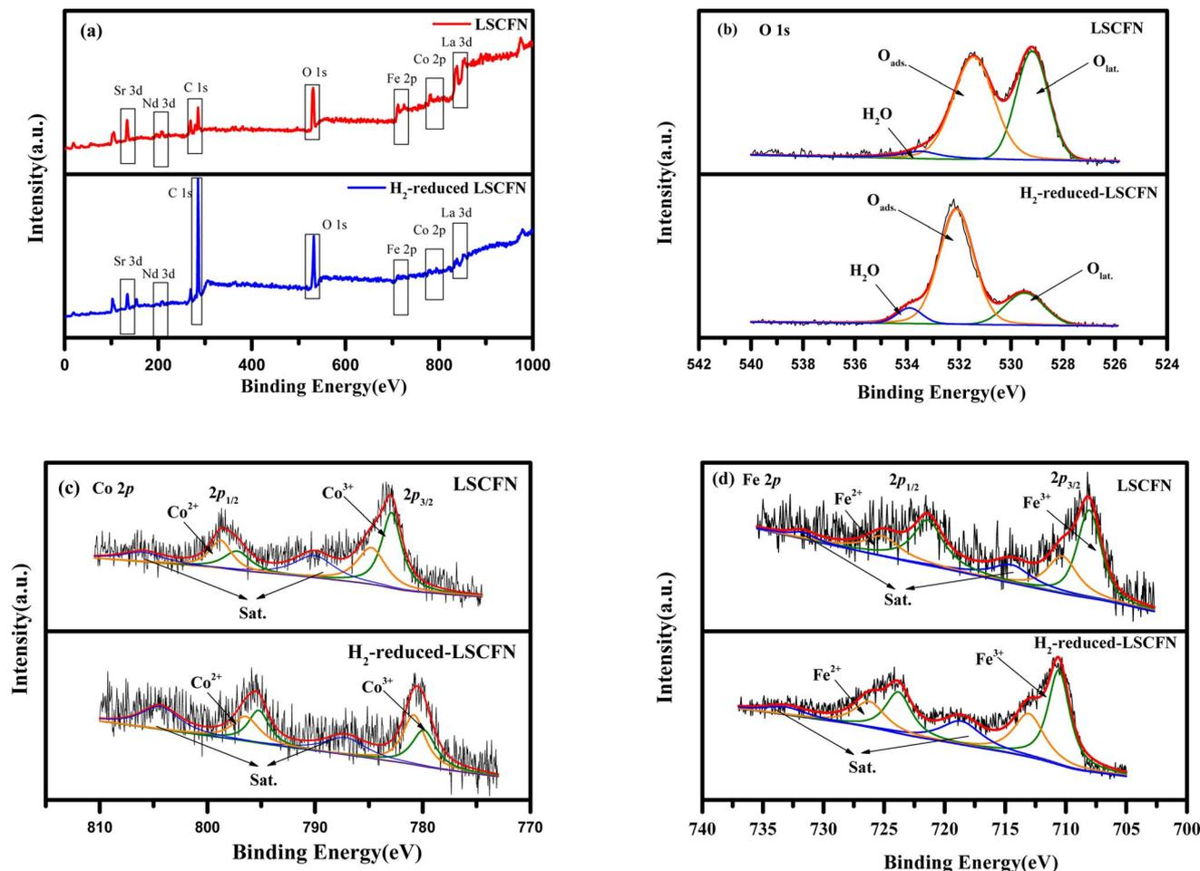
Fig. 2 XPS survey spectra (a), O 1s XPS spectra (b), Co 2p XPS spectra (c), and Fe 2p XPS spectra (d) of LSCFN and H<sub>2</sub>-reduced LSCFN samples.
