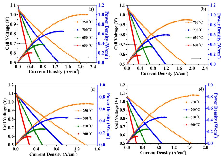
Fig. 6 The *I-V-P* spectra of cathode-impregnated (a) and full cell impregnated (b) MSCs under H<sub>2</sub> atmosphere, and the *I-V-P* spectra of cathode-impregnated (c) and full cell impregnated (d) MSCs under CH<sub>4</sub> atmosphere.
