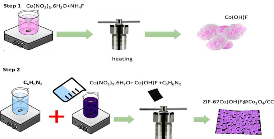
Fig. 1 Schematic diagram of ZIF-67Co(OH)F@Co<sub>3</sub>O<sub>4</sub>/CC synthesis.
