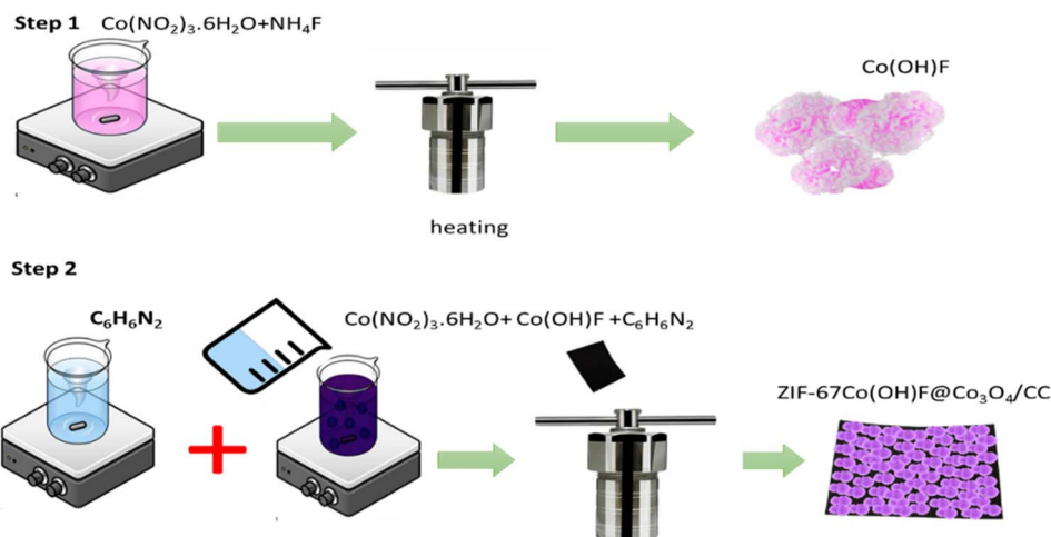
Fig. 1 Schematic diagram of ZIF-67Co(OH)F@Co 3 O 4 /CC synthesis.
